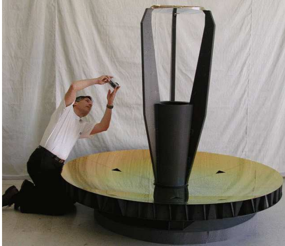
Figure 2.16.1: The COI mirror assembly
