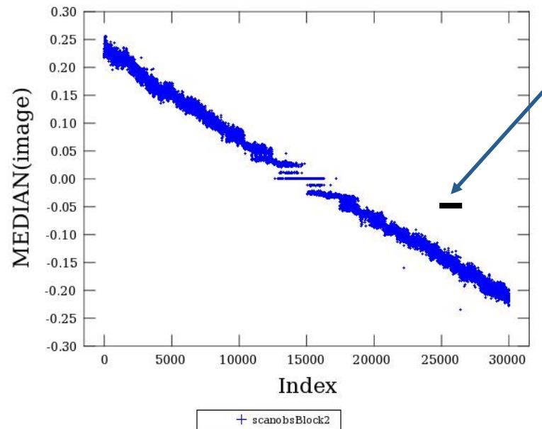
*Divide the array median in bins of  $N$  readouts.  $N$  is typically 1000 readouts.*
