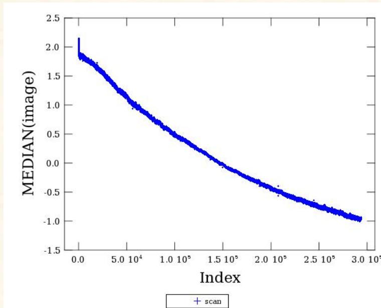
*This Figure illustrates what is meant by both correlated and drift for PACS signal. The Figure shows the median value of the bolometer array as a function of readout index. The monotonic signal showing a decay in intensity is commonly observed in PACS' image cubes, and is thought to be related to focal plan temperature drifts.*
