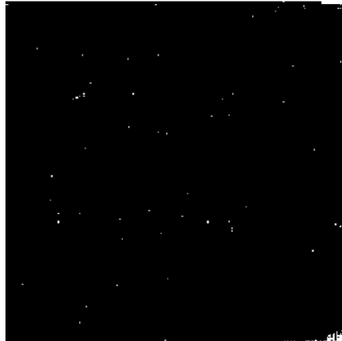
Figure 51 The relatively clean LWC bad pixel mask from OC9P that changed little over time.
