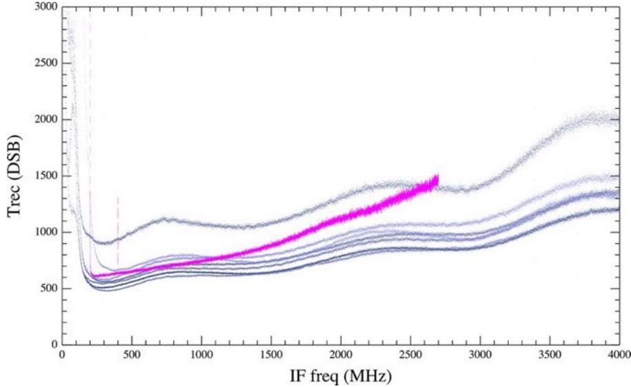
**Figure 10** LFAH receiver temperature curves from [Risacher et al. \(2016\)](#) for all seven pixels in the array. The purple line is the single-pixel L2 receiver for comparison.
