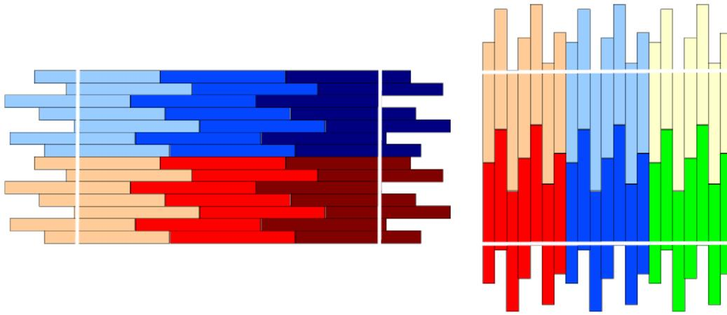
Figure 7. A single map could consist of any number of blocks and could scan in the x- or y-direction or both. Occasionally overlapping scans were done in both directions to minimize striping effects caused by the different characteristics of individual array pixels.
