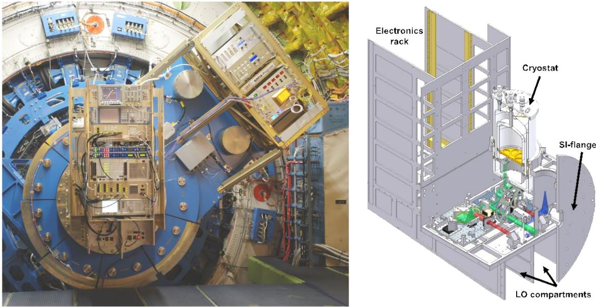
**Figure 2** From *Heyminck et al. (2012)*. (Left) Image of GREAT mounted on the SOFIA instrument flange. The components of the instrument are mounted on the end of the flange seen near the center of the image, while the backend is mounted on the counterweight in the upper right of the image. (Right) Diagram showing the GREAT components mounted on the end of the flange.
