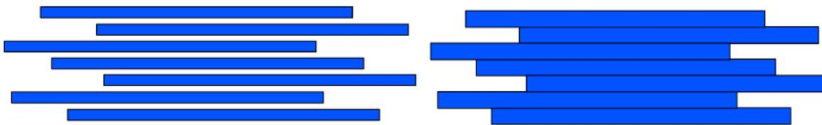
**Figure 6** (Left) Example of a block with a single scan. The gaps between the scanned pixels indicate an under-sampled map. (Right) Example of a block with two scans. This block is fully sampled in the direction perpendicular to the scan direction. The second scan fills in the gaps in the single-scan block.
