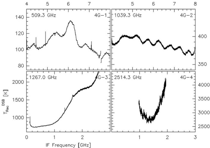
**Figure 12** *4GREAT receiver temperature curves from Durán et al. (2020) for the four 4GREAT channels.*
