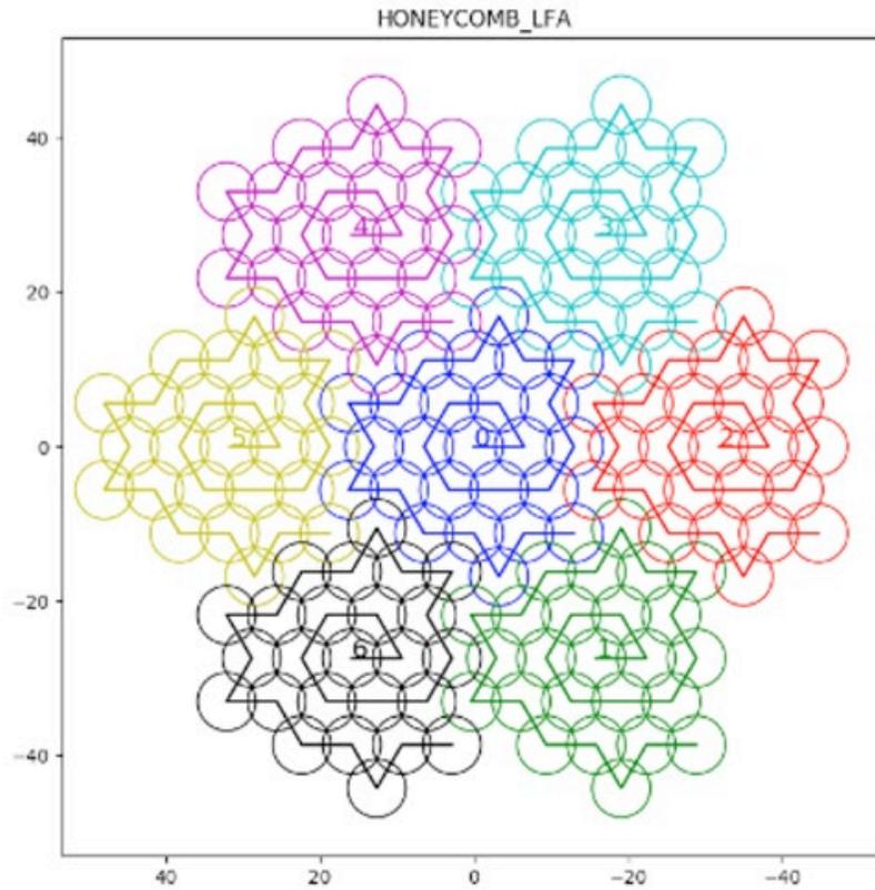
**Figure 8** Example Honeycomb pattern for the LFA with all pixels showing how the pointings mesh together. Each color represents a separate pixel in the array, and the line shows the motion of the scan. The units of the axes are in arcseconds. The pattern for the HFA was a factor of  $2.7\times$  smaller since the pattern scales with the array size.
