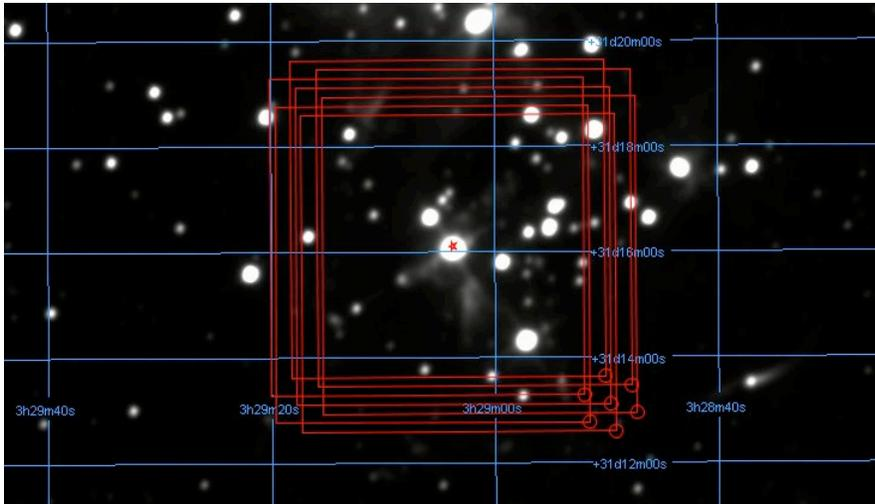
**Figure 4** Example overlay of a Classical OTF map for the LFA. Each red rectangle shows the region mapped by one of the LFA pixels. The footprint of the array is shown by the red circles on the bottom right and marks the starting position of the map. The central region of the map is covered once by each pixel of the array.
