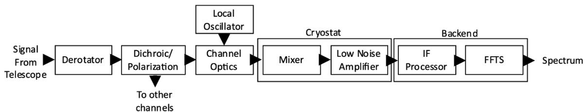
**Figure 3** Chart for GREAT showing how the signal from the telescope passed through each component of the instrument for a single channel before finally ending up as the Level 1 data. This chart is based on Figure 3 in *Risacher et al. (2018)*.
