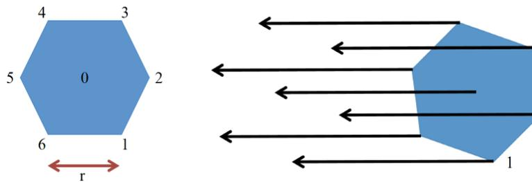
**Figure 5** Array configuration and an illustration of how a rotation of the array of 19.1 degrees allows equidistant scans.
