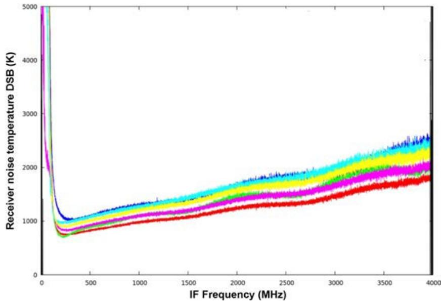
**Figure 11** HFA receiver temperature curves from [Risacher et al. \(2018\)](#) for all seven pixels in the array.
