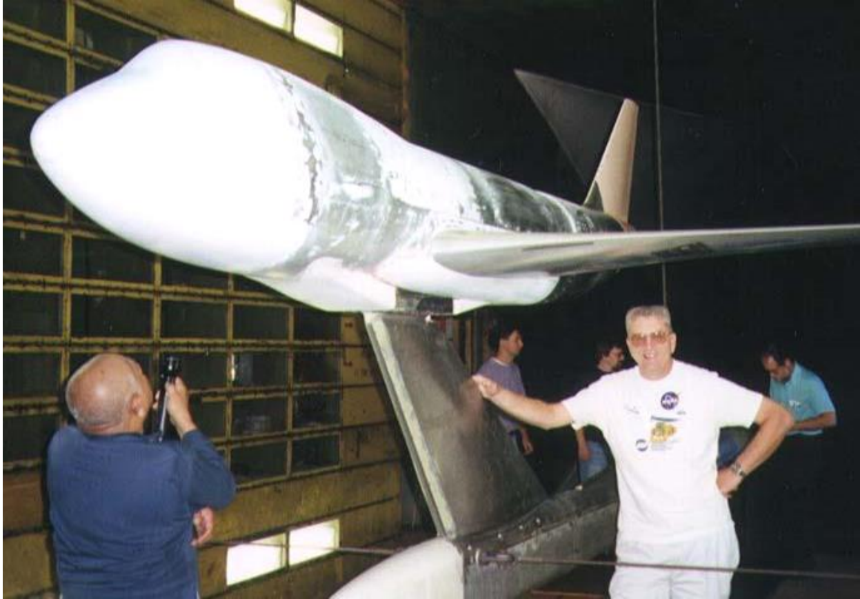
Figure 5.2-3. Dr. Bill Rose with the SOFIA 7 percent wind tunnel model used to develop SLC design technology and determine cavity acoustic environment and resultant loads on the telescope in the test section of Ames' 14-ft Transonic Wind Tunnel.
