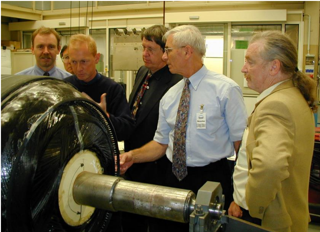
Figure 7.5-10. The SOFIA Nasmyth tube being made via a filament winding process at MAN – September 19, 2000.
