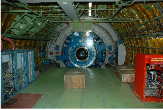
Figure 7.11-6. Inside looking aft towards the installed telescope.
