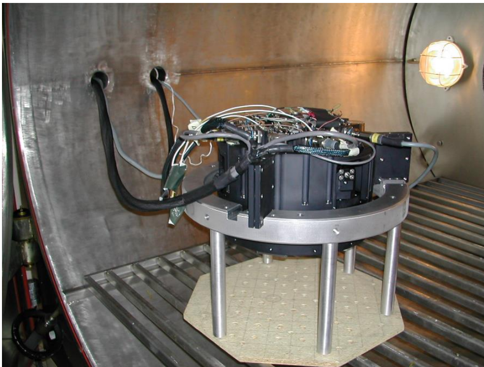
Figure 7.8-11. Meanwhile in Austria environmental test facilities, the secondary mirror mechanism was being tested again to make sure it would work properly at the extreme temperature environment that it would experience during operations – March 2003.
