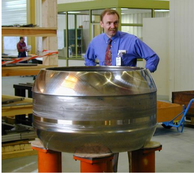
Figure 5.4-2. That's me standing behind the 1.2-meter diameter RIS sphere that supports the floating part of the telescope and is the key component that isolates the telescope from aircraft rotations.
