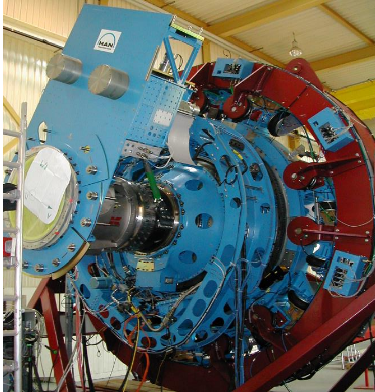
Figure 7.7-26. The cabin side of the TA, near completion of pre-ship integration within the dummy bulkhead (the red structure) at MAN in Augsburg, Germany – July 12, 2002.
