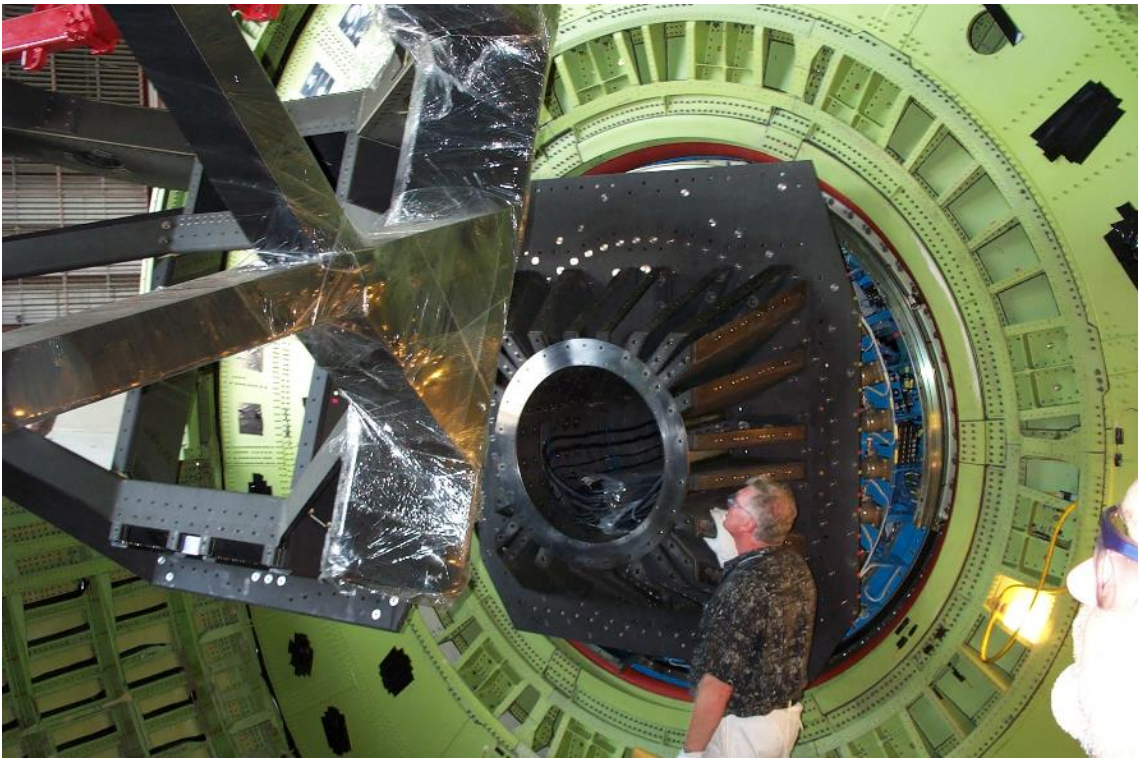
Figure 7.8-17. The telescope metering structure getting close to the SUA attachment interface in the aircraft cavity – May 2, 2003.
