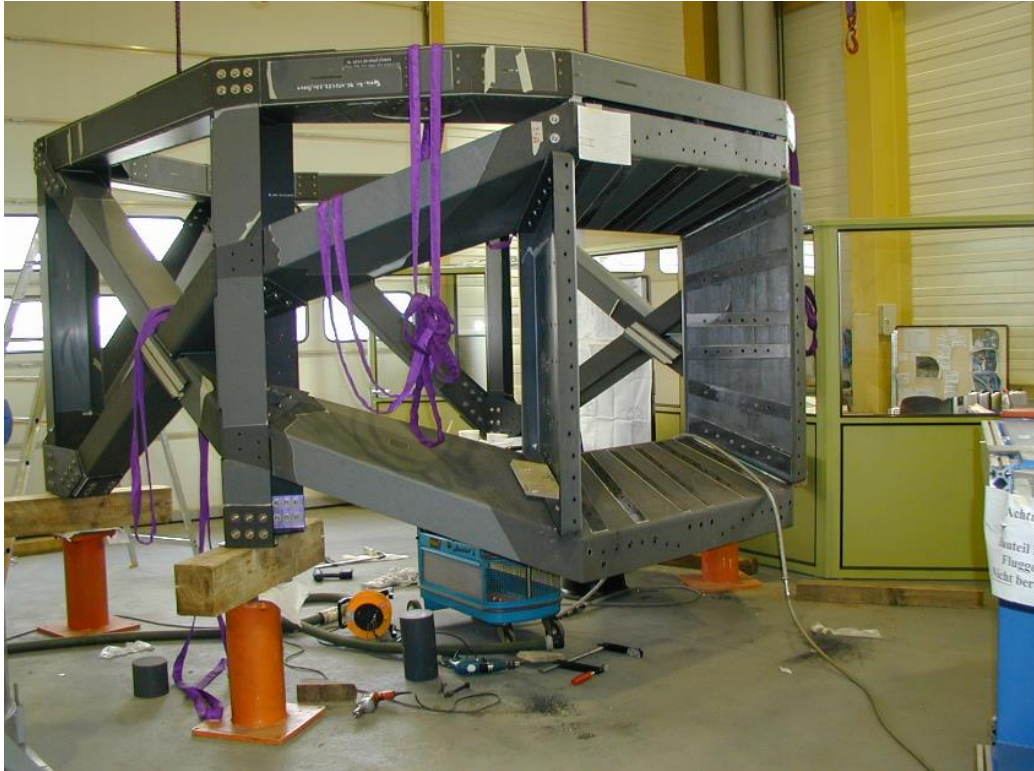
Figure 7.6-14. Composite metering structure.
