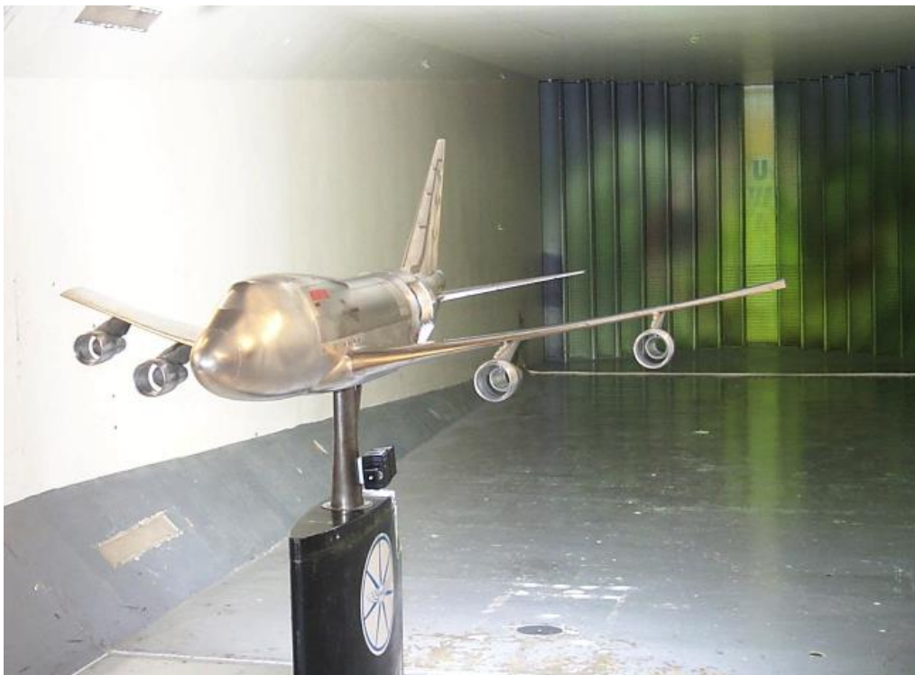
Figure 5.2-5. The 3-percent SOFIA Model in Kirsten Wind Tunnel.
