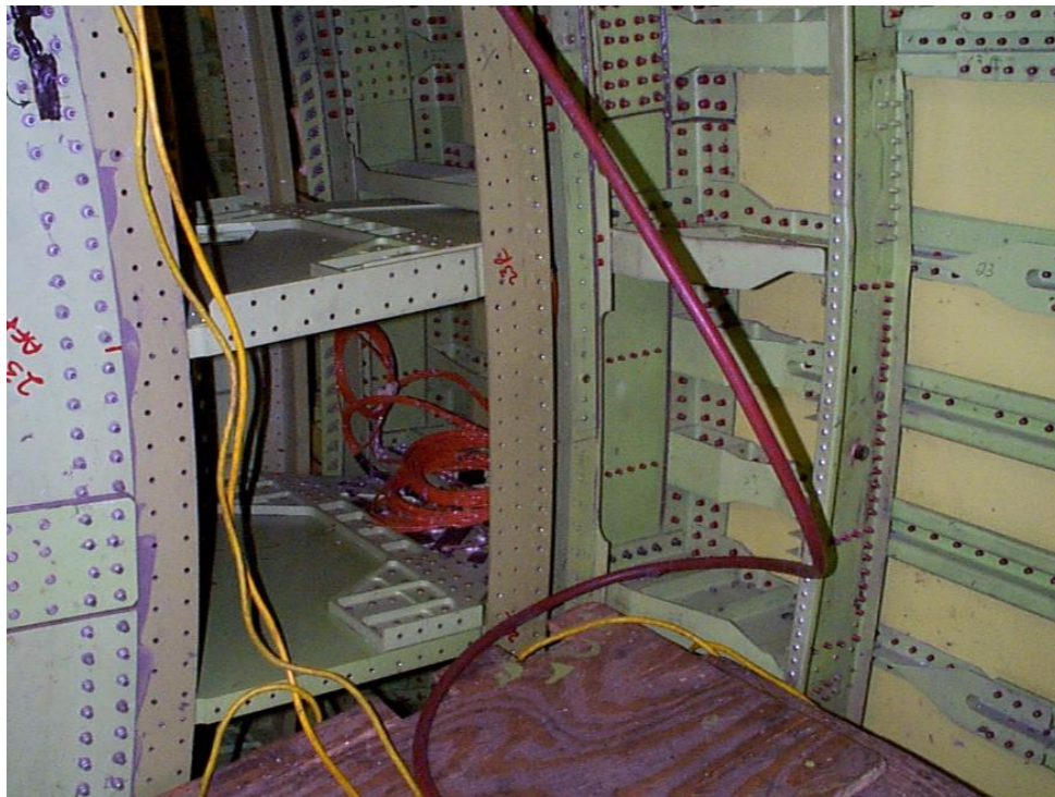
Figure 7.7-48. The pin joint pressure bulkhead being installed into the aircraft – November 2002.
