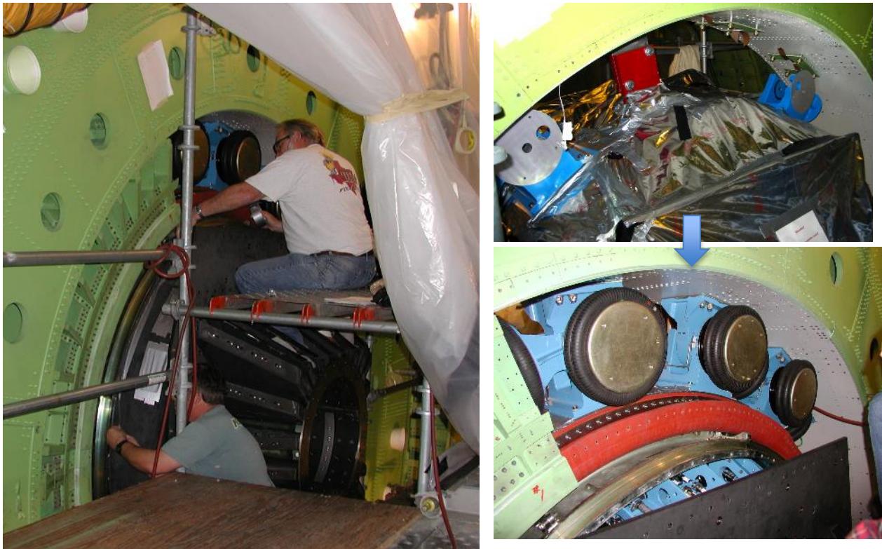
Figure 7.8-9. The SUA installation continuing with NASA Ames Technicians John Wallace and Ron Strong helping out our German colleagues installing the VIS and related hardware that attaches the telescope to the aircraft – February 2003.
