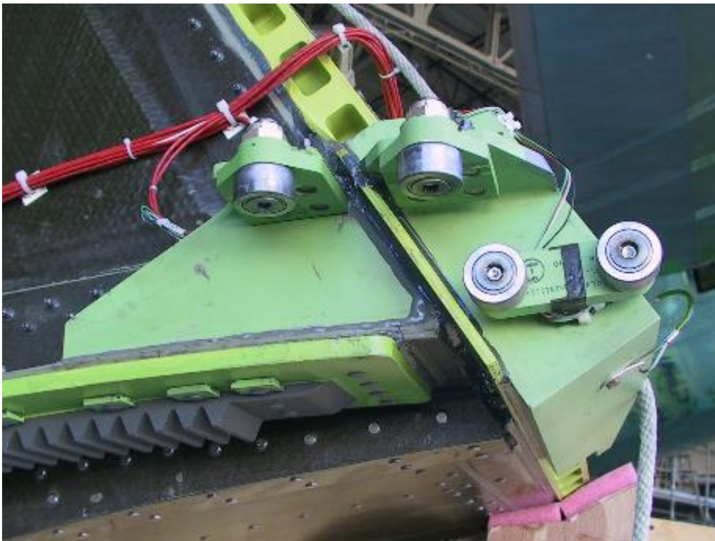
Figure 7.10-3. Just a small sample of multiple sets of mechanisms that enable precise cavity door motion while accommodating the flexibility of the 747 fuselage structure.
