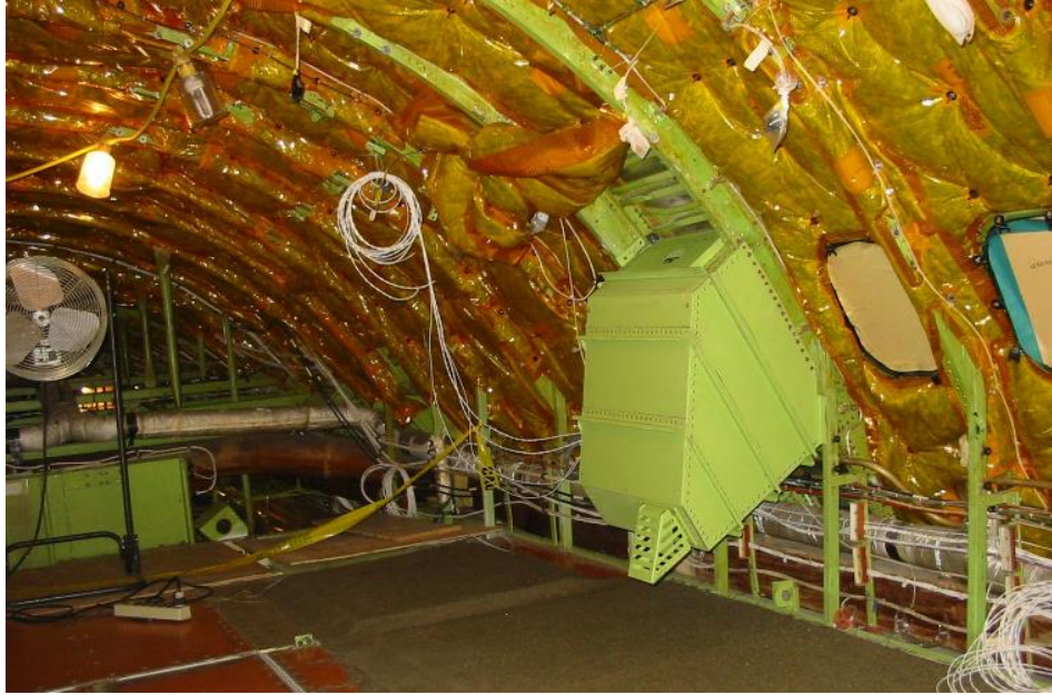
Figure 7.8-32. Looking aft in the upper deck of SOFIA, showing the Water Vapor Monitor installed onto one of the former window locations – September 19, 2003.
