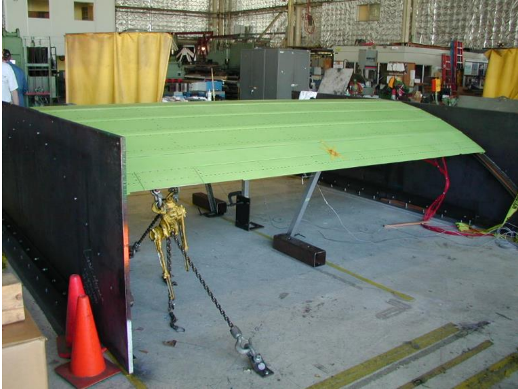
Figure 7.8-12. Also in March, back at Ames, the Lower Flex Door (LFD) was being tested with sandbag weights to verify the structural integrity under predicted worse case loading – March 2003.
