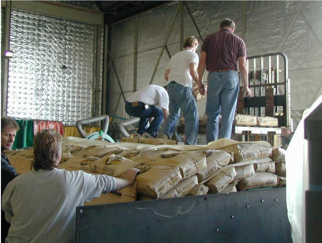
Figure 7.8-14. The LFD with three layers of the 70-lb sandbags loading the structure with both the engineers and technicians handling load – March 2003.
