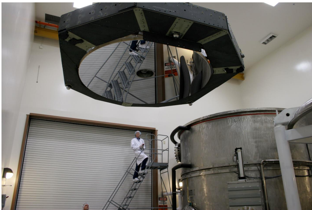
Figure 8.1-3. The SOFIA primary mirror gets coated for the first time, in the mirror coating facility at NASA Ames Research Center – July 2008.
