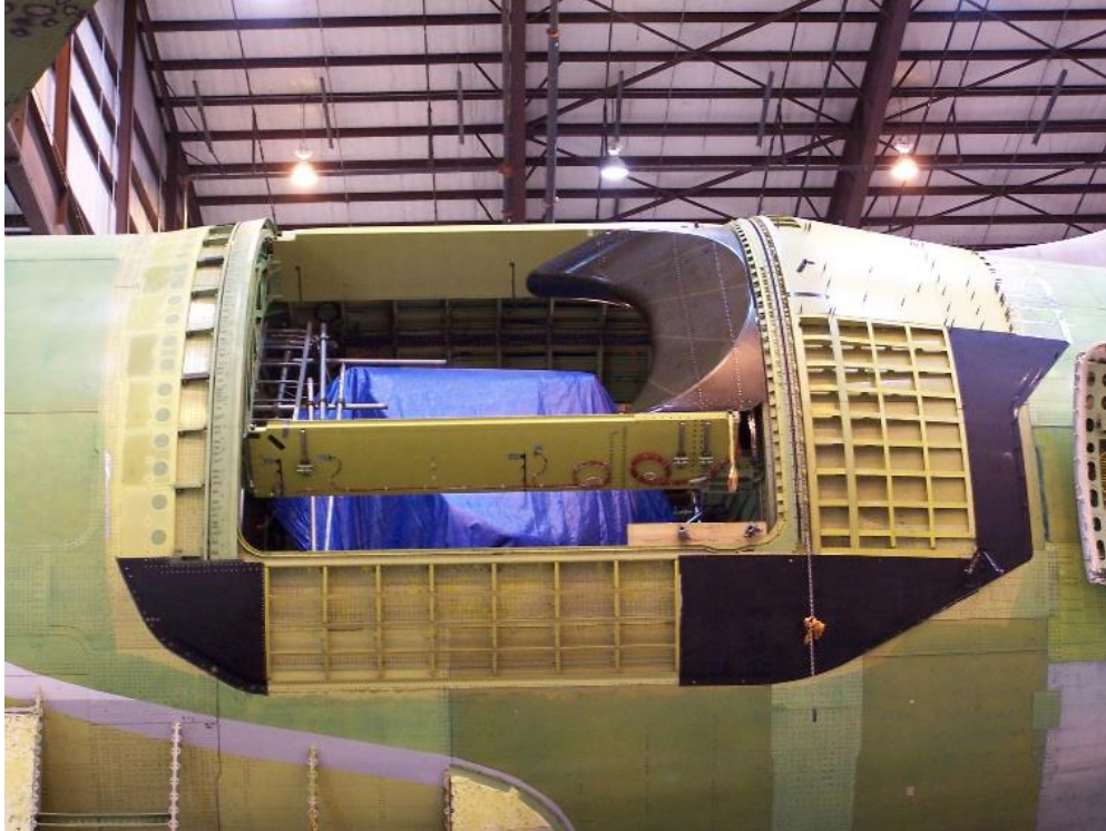
Figure 7.10-5. Cavity Door Aperture in place showing the aft ramp that we developed for SOFIA to catch the airstream-shear layer and provide a quiet cavity environment for the telescope during open-door flight.
