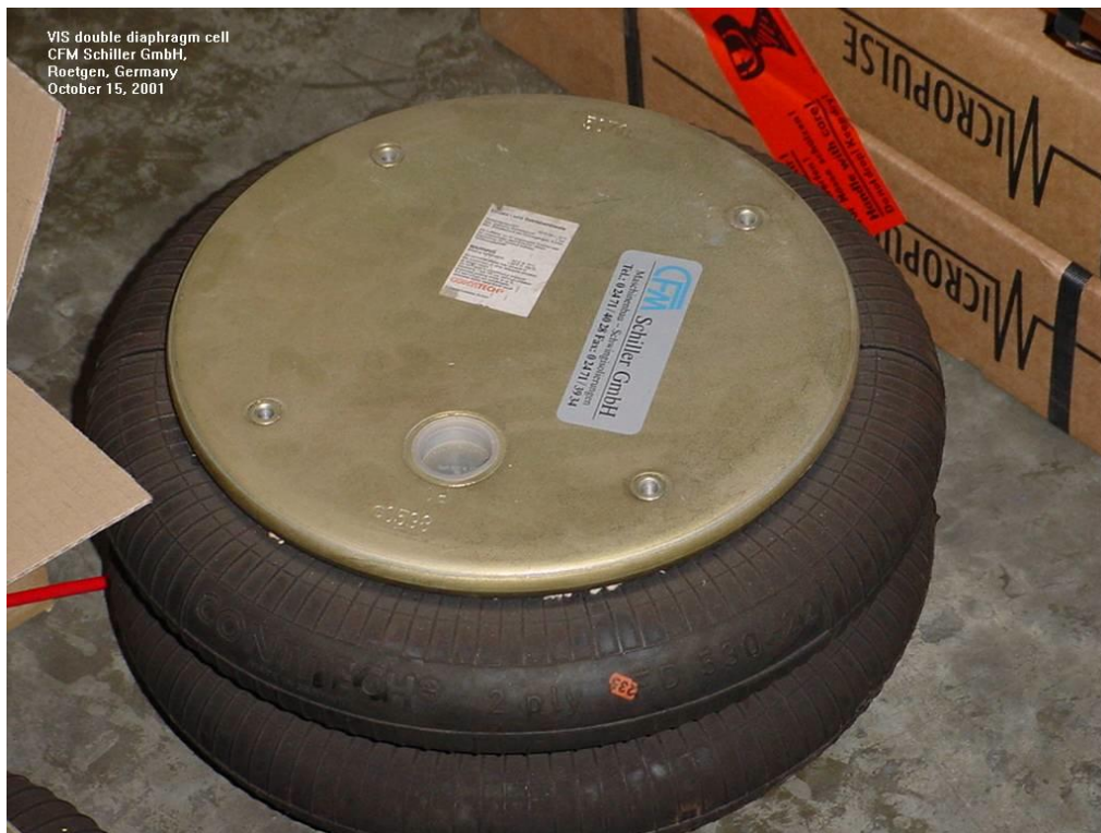
Figure 7.6-28. One of the dual diaphragm VIS components.
