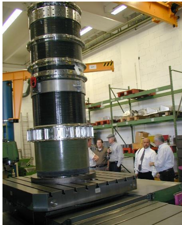
Figure 7.6-11. The carbon fiber Nasmyth tube almost ready to begin integration. At MAN in Augsburg, Germany – June 2001.
