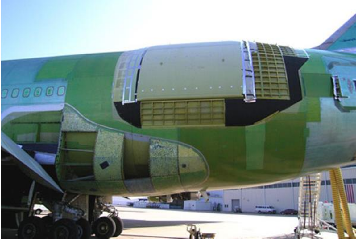
Figure 7.10-9. Cavity door system mostly installed – October 20, 2005.
