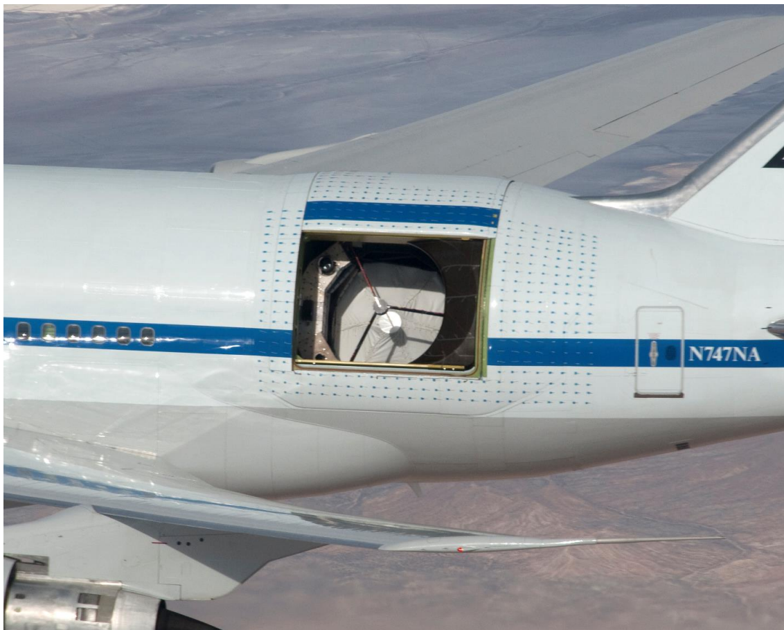
Figure 8.1-7. A close-up of the cavity area, during open door flight testing. Note the cover over the mirror – 2009.
