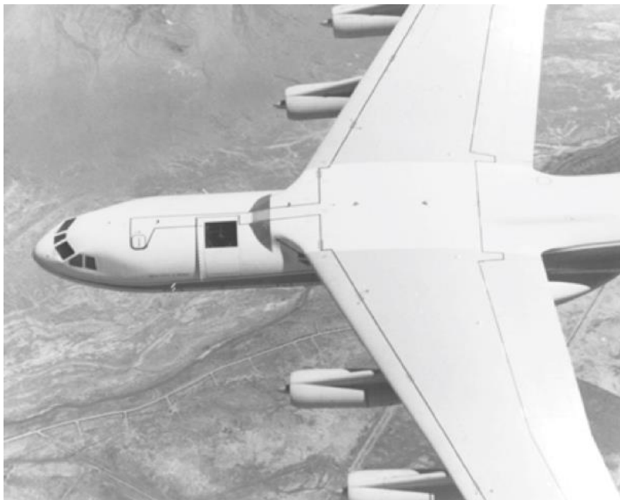
Figure 4.0-2. View looking down on the open port cavity of the KAO in flight.
