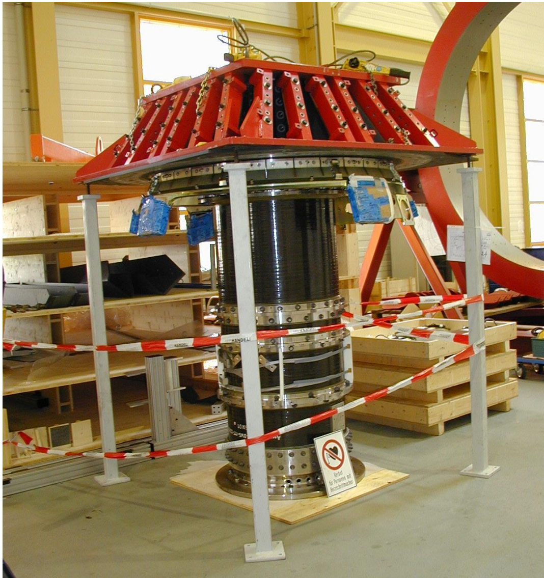
Figure 7.6-21. The Nasmyth tube ready to be inserted into the RIS inner SUA – late September 2001.
