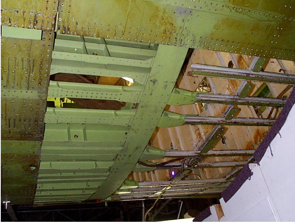
Figure 7.6-16. The old skin being removed from the belly of the aircraft, Waco, Texas – July 2001.
