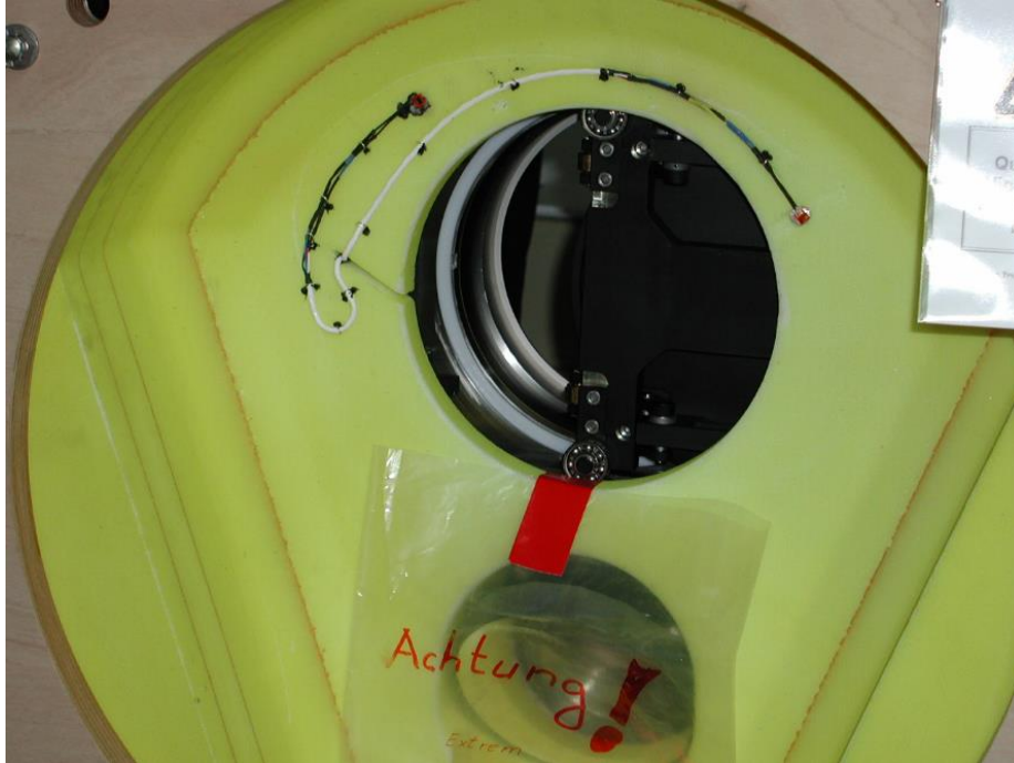
Figure 7.7-8. The inside of the SI flange assembly, showing the gate valve and the path to the FPI.
