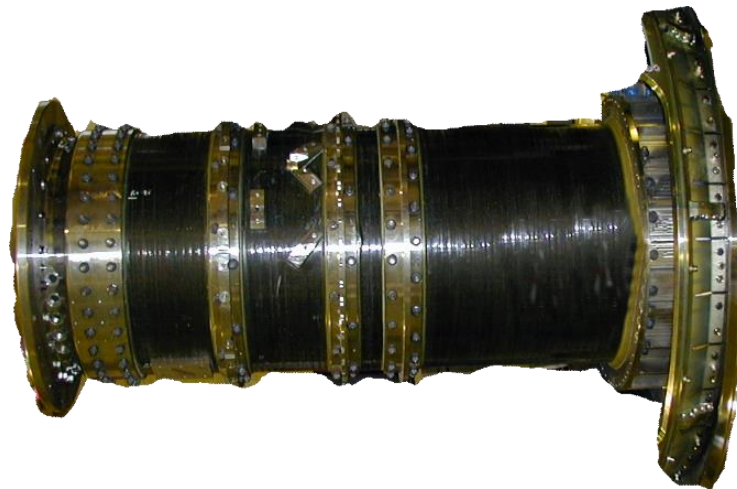
Figure 5.4-5. The carbon fiber filament-wound Nasmyth tube that connects the telescope metering structure in the cavity to the SI in cabin supports both sides on the RIS.
