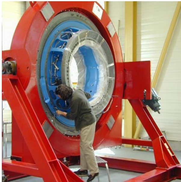
Figure 5.4-3. Dr. Jackie Davidson checking out the inner suspension assembly (SUA) where the RIS sphere will soon be installed.
