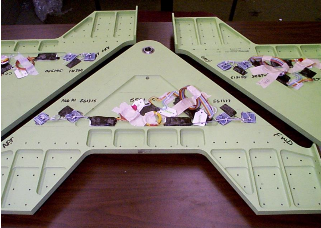
Figure 7.7-34. The bulkhead to fuselage attachment structures. A pinned joint.
