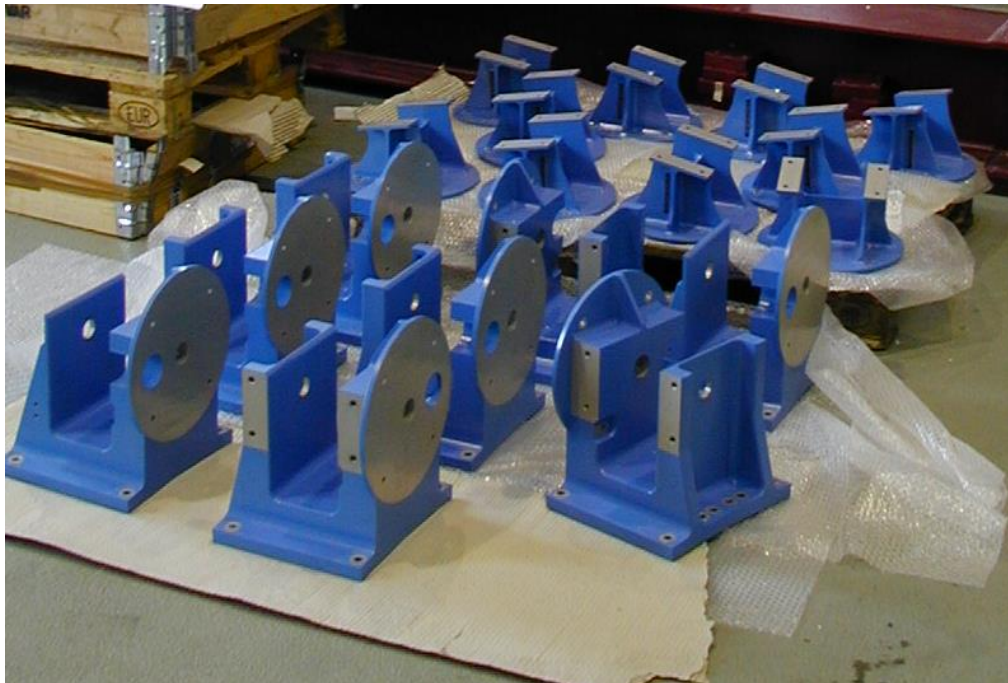
Figure 7.6-39. The VIS brackets that attach the telescope to the aircraft or dummy bulkhead.
