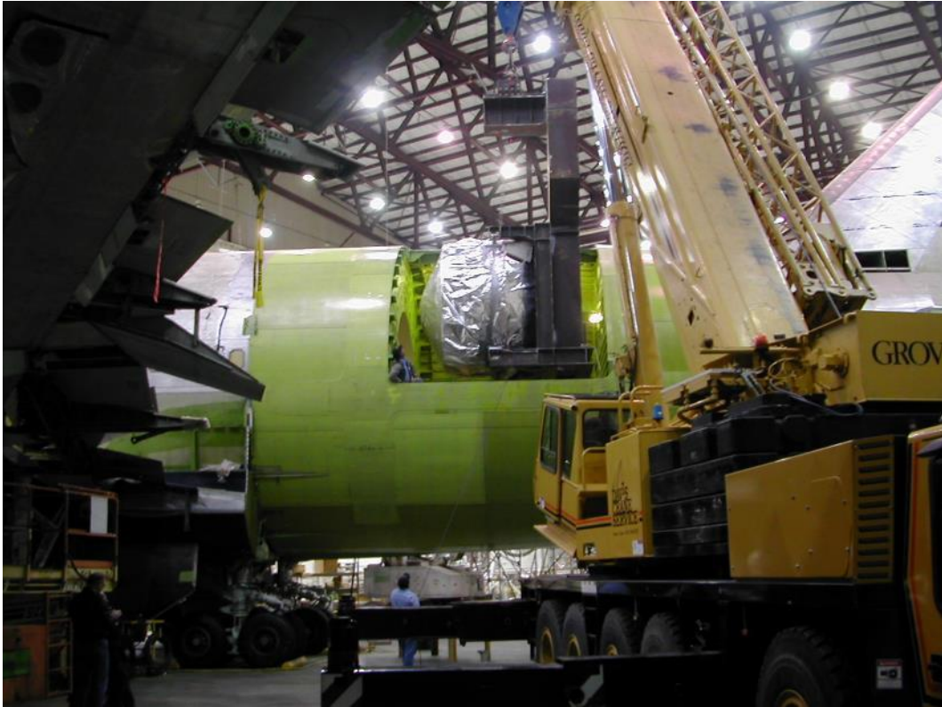
Figure 7.8-6. Lowering SUA into cavity – January 2003.
