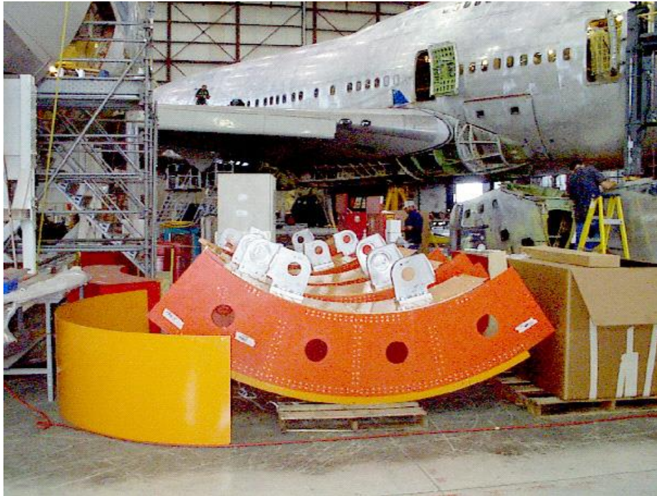
Figure 7.4-1. The prototype bulkhead segments with simulated VIS brackets about to be installed into the scrap section 46 (upper left of photo) to practice/evaluate installation procedures – Waco, July 1999.
