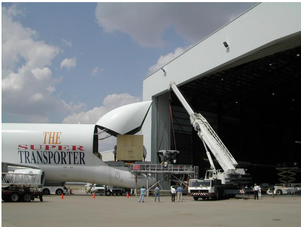
Figure 7.7-41. Unloading the large SOFIA telescope components from the Beluga into the hangar where the SOFIA aircraft was located.
