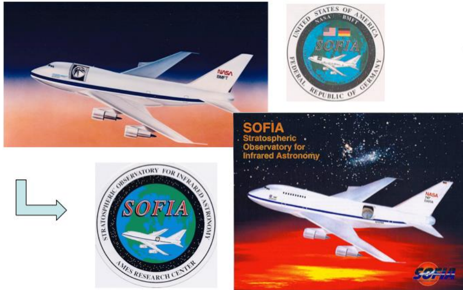
Figure 6.10-1. Shows the changes in the artist concepts and SOFIA sticker when the cavity was moved from the front to the back.
