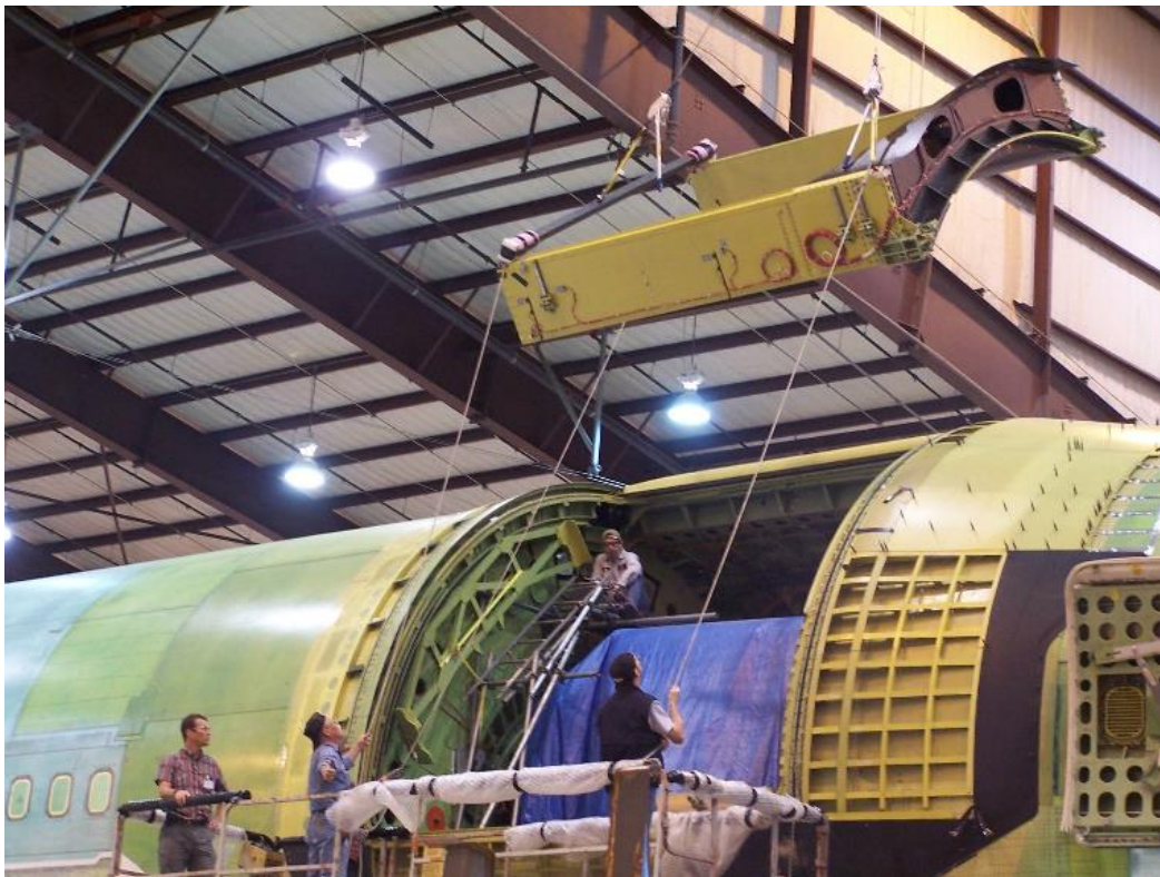
Figure 7.10-4. Cavity Door aperture being installed – February 2005.
