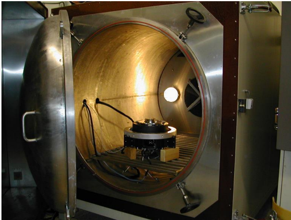
Figure 7.7-50. The Secondary Mirror Mechanism being tested in the thermal chamber – December 2002.
