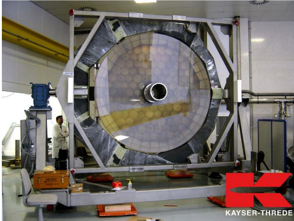
Figure 7.7-28. The uncoated primary mirror mounted within the CFRP mirror cell, attached to a fixture in preparation to be shipped.
