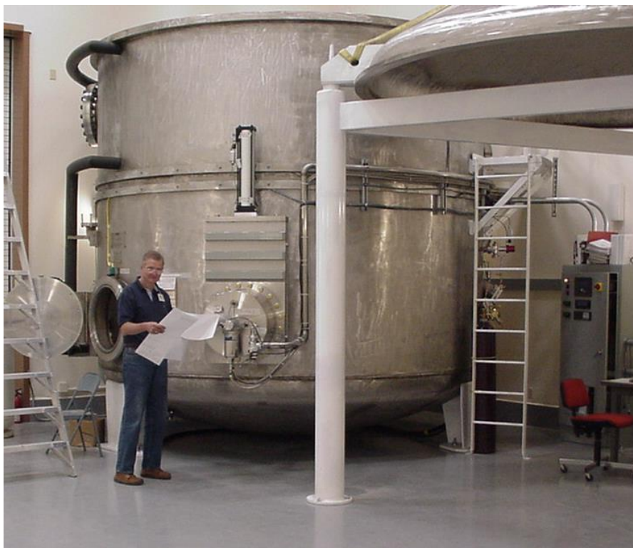
Figure 7.6-5. The mirror coating facility vacuum vessel inside the Hangar N211 at NASA Ames Research Center – April 2001.
