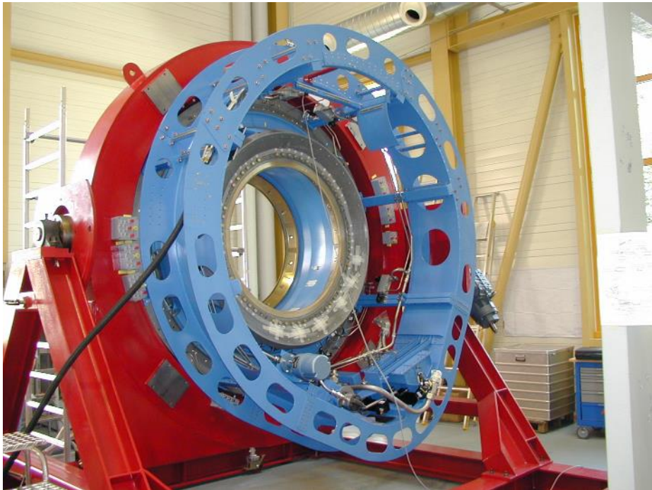
Figure 7.6-13. The inner SUA with the 1.2-meter-diameter spherical socket ready to for 1.2-meter-diameter RIS (photo shown in telescope engineering highlights section).
