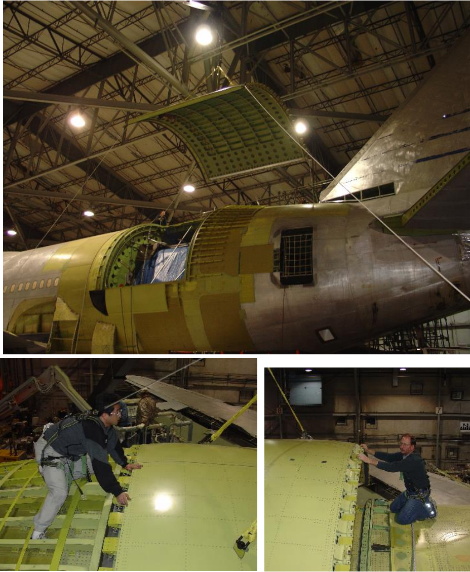
Figure 7.9-14. NASA Ames engineers Glenn Sasaki and Fred Martwick helping install the partial external door – December 2004.
