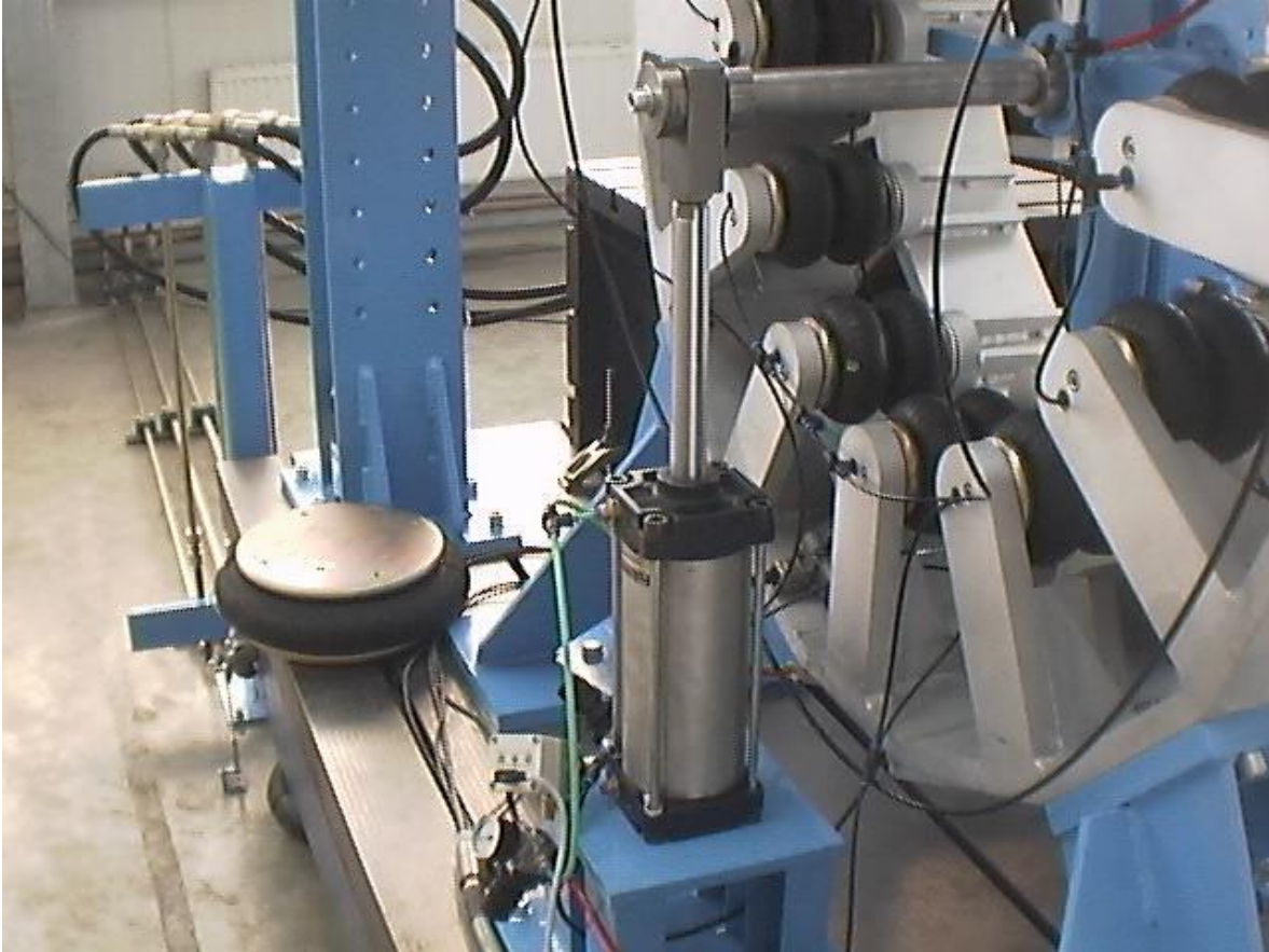
Figure 7.4-3. The air bladder components of the TA VIS being tested.
