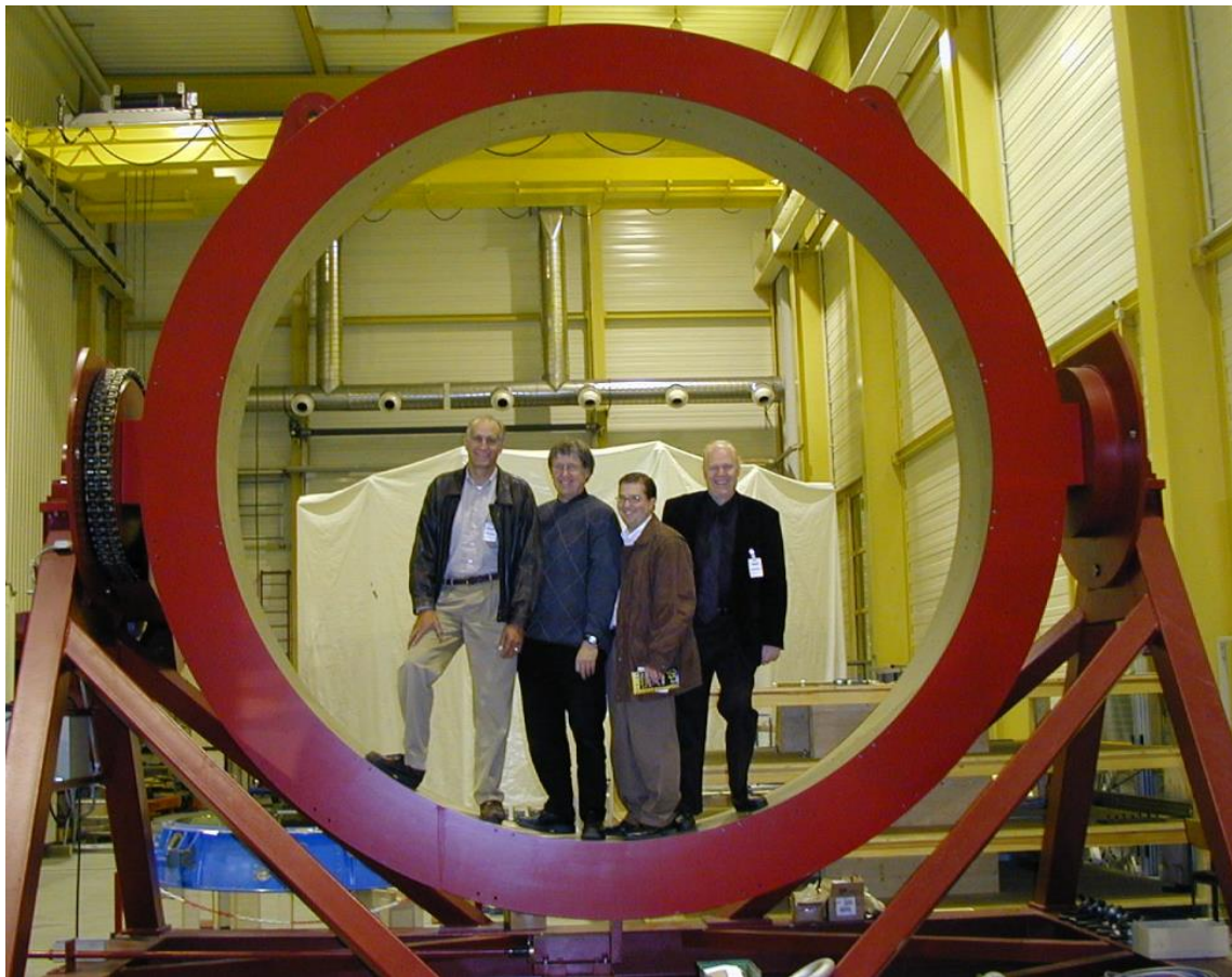
Figure 5.3-7. Cliff Imprescia, Hans Kaercher, John Fitch and Eric Becklin in the bulkhead simulator used to build up the telescope assembly (TA).
