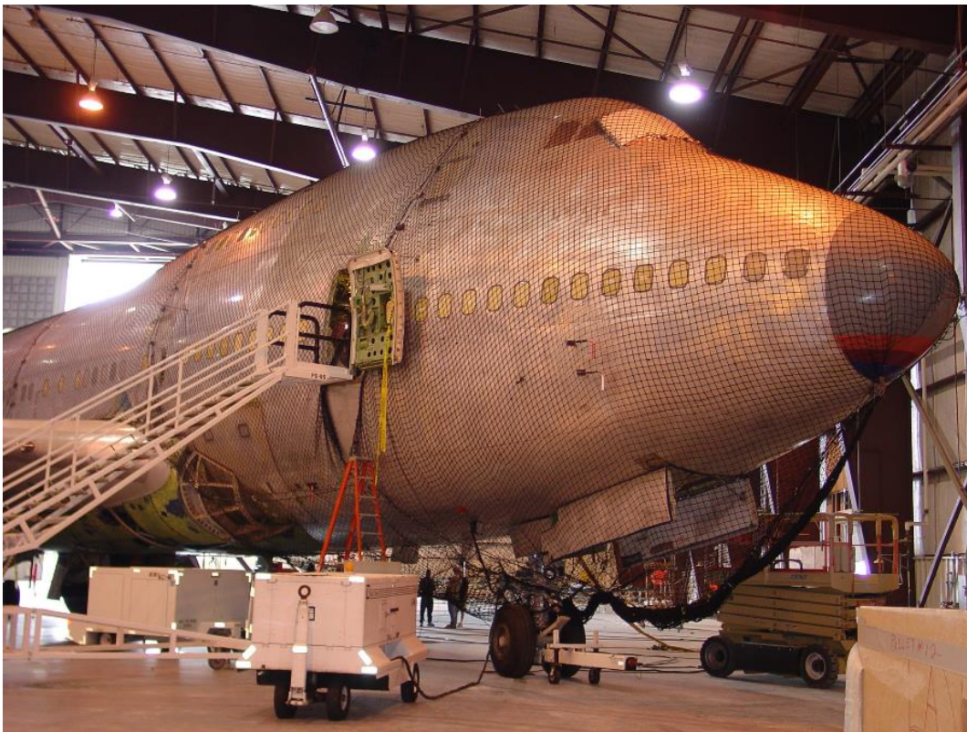
Figure 7.9-6. The aircraft shortly before starting the proof pressure test with a net to provide some safety/containment in case of structural failure.
