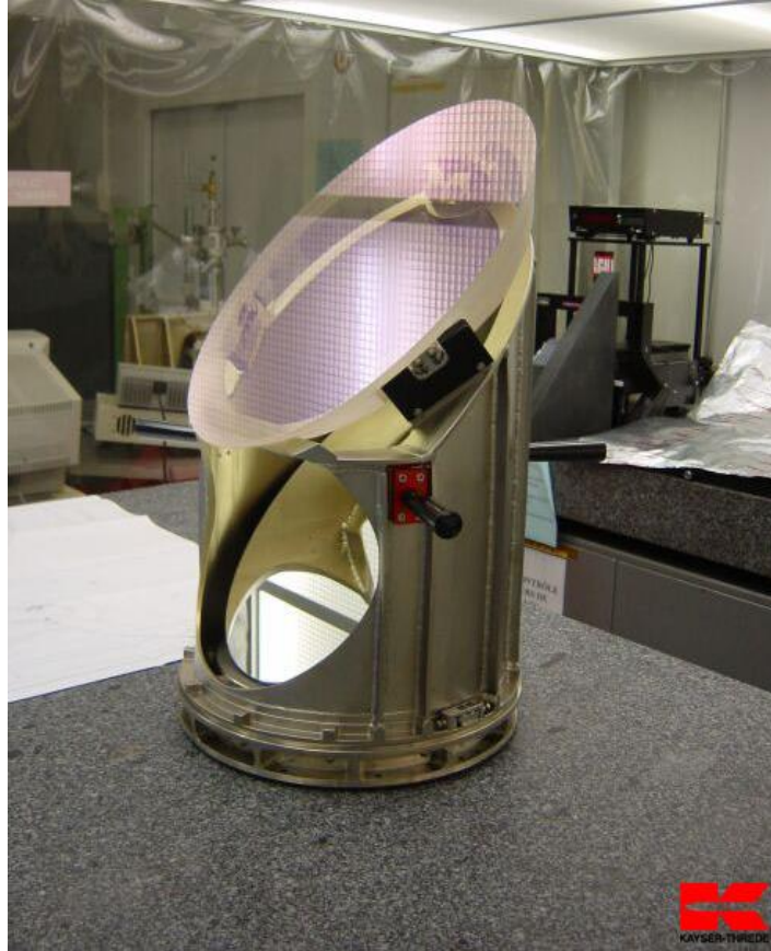
Figure 5.4-17. Dichroic tertiary mirror on tower with visible light reflecting mirror.
