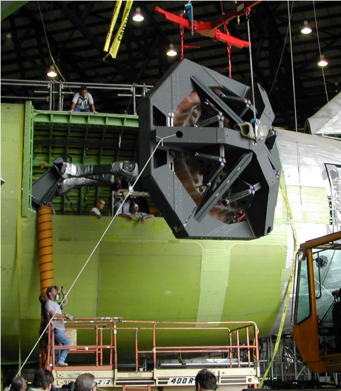
Figure 7.8-24. Primary Mirror installation – July 15, 2003.
