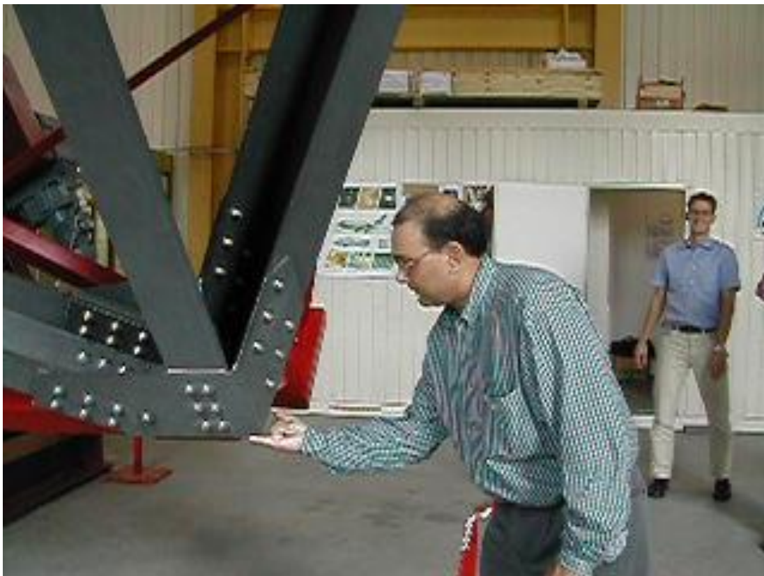
Figure 5.5-4. A clip from the video showing Kaiser Adeni being able to move about 18,000 lbs of the floating telescope with his pinky finger because the RIS works so well.
