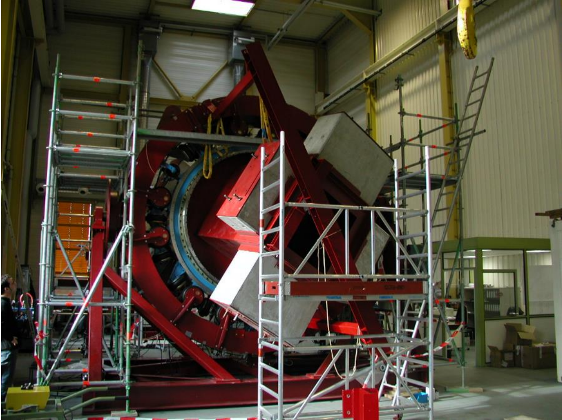
Figure 7.7-12. The outer SUA or SUA III, with a mass/inertia simulator to measure, adjust and optimize performance of the VIS and damping system – March 5, 2002.
