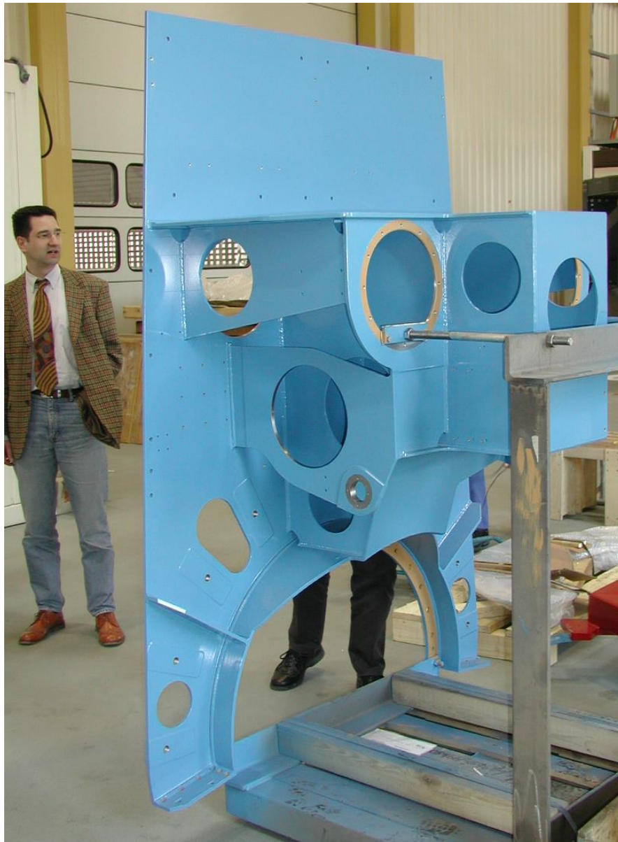
Figure 7.7-18. The counter-weight weldment ready to be installed onto the cabin side of the SUA with Eckhard Bremers – April 2002.
