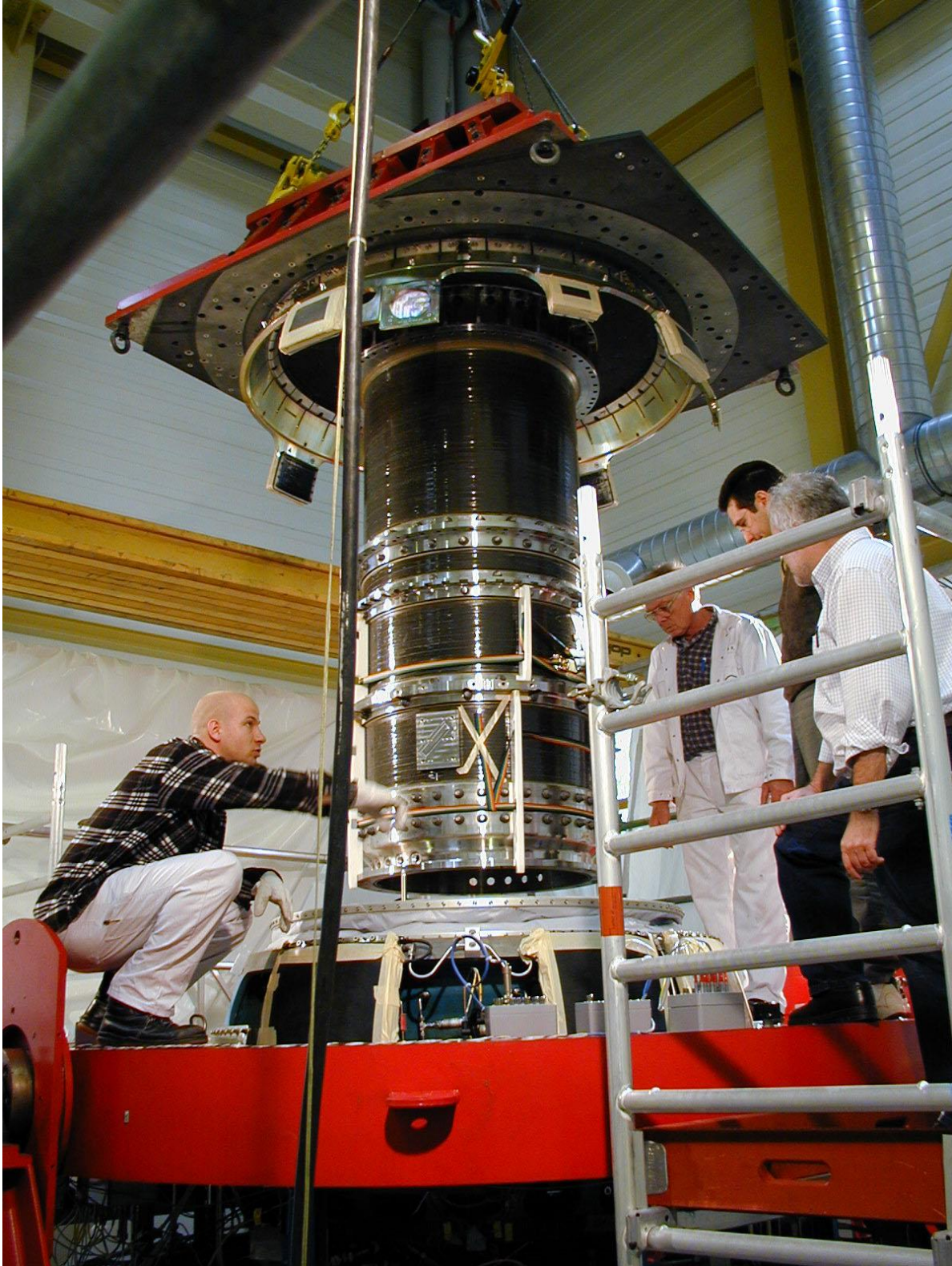
Figure 7.6-22. Installation of the Nasmyth tube into the RIS/Inner SUA – September 26, 2001.
