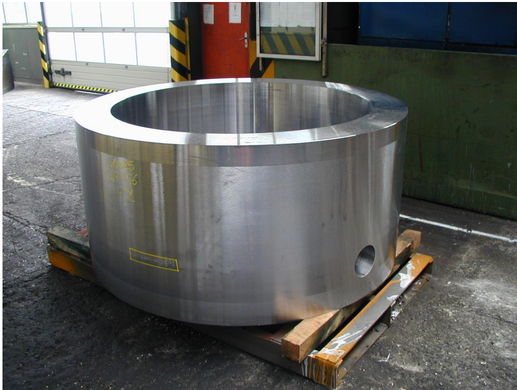
Figure 7.5-5. The large piece of steel that the TA inner cradle will be made from – May 31, 2000.
