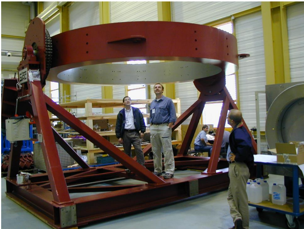
Figure 7.6-26. L3's John Fitch and I checking out the dummy bulkhead in Augsburg that was used to assemble and integrate the SOFIA telescope for the first time.
