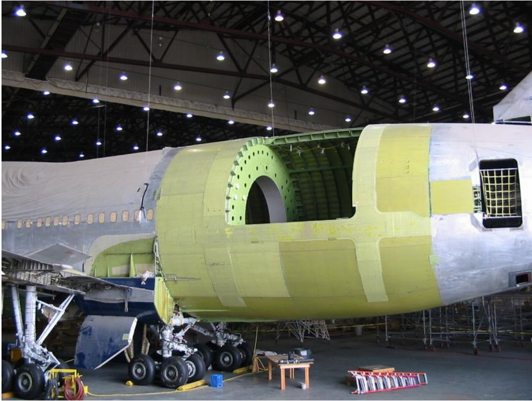
Figure 7.8-4. The aircraft modification almost ready to begin installing the TA – January 2003.
