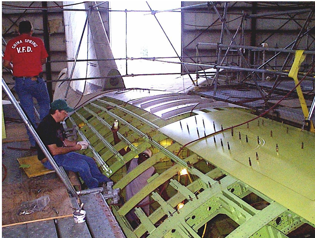
Figure 7.7-36. Status of the aircraft modification, re-skinning-re-enforcement – August 15, 2002.
