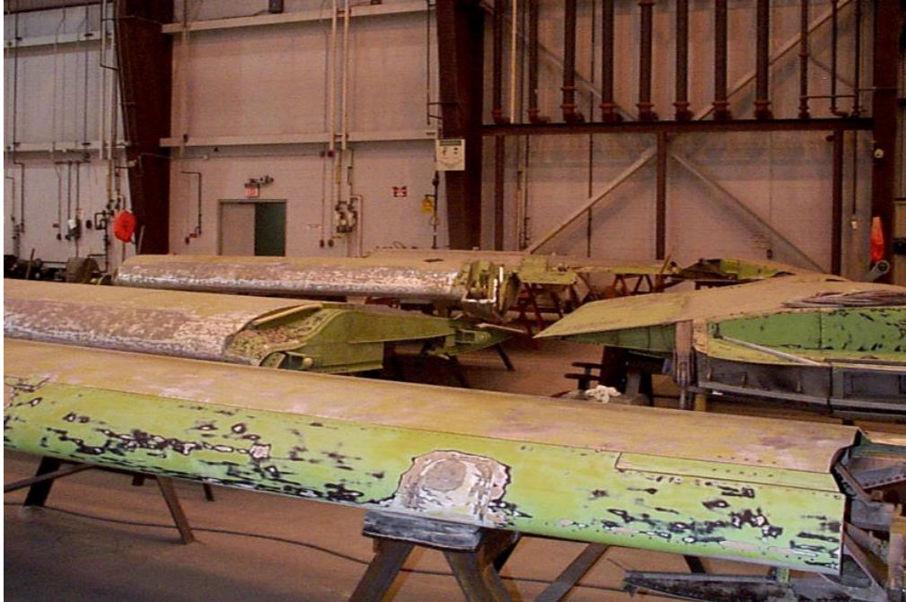
Figure 7.9-3. Aircraft control surface components being refurbished and prepped to be painted – April 2004.
