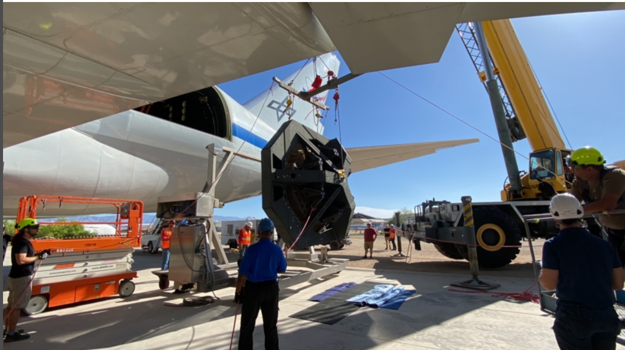
Primary Mirror Assembly being removed from the SOFIA aircraft. Credit: DSI/Florian Behrens
