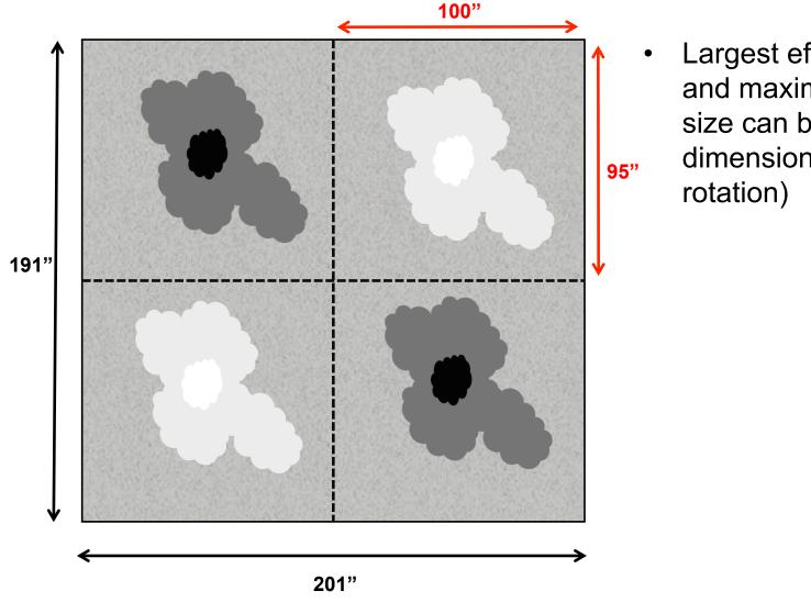
Largest effective FoV and maximum source size can be 95" (smallest dimension because of rotation)
