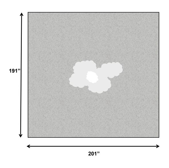
With no chopping, source would be located on center of frame at the telescope optical axis
