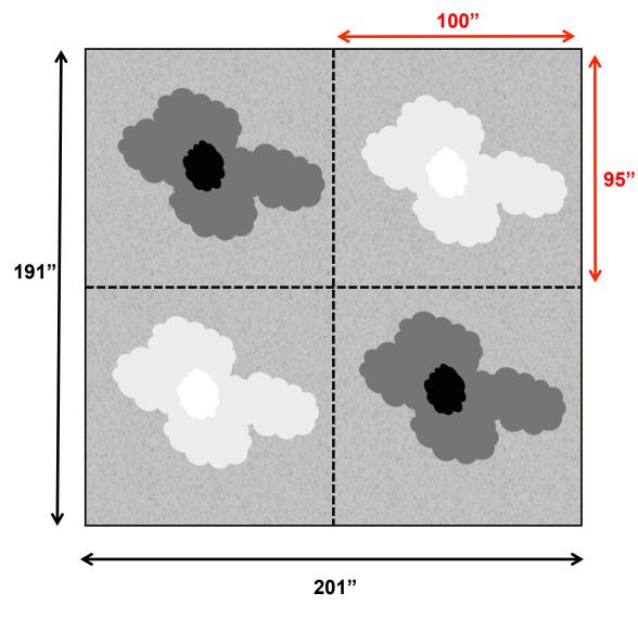
Largest effective FoV and maximum source size can be 95" (smallest dimension because of rotation)
