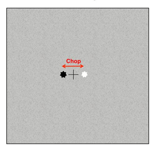
If you turn on the chopper the mirror would back and forth about the telescope optical axis
