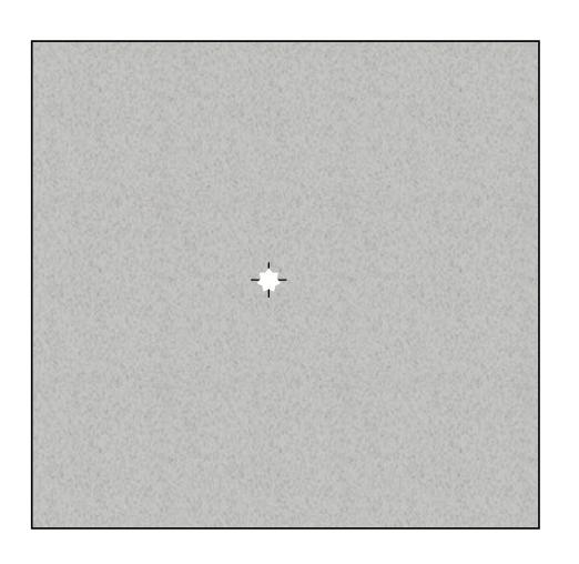
With no chopping, source would be located on center of frame at the telescope optical axis
