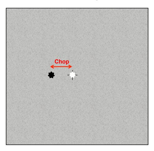
In this case, the mirror moves between the optical axis and an offaxis position
