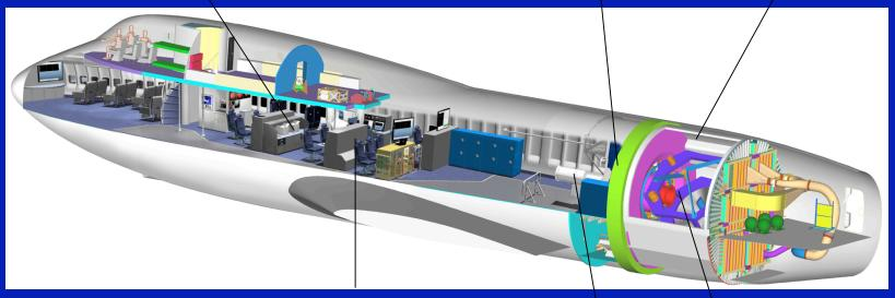
scientist stations, telescope and instrument control, etc.
