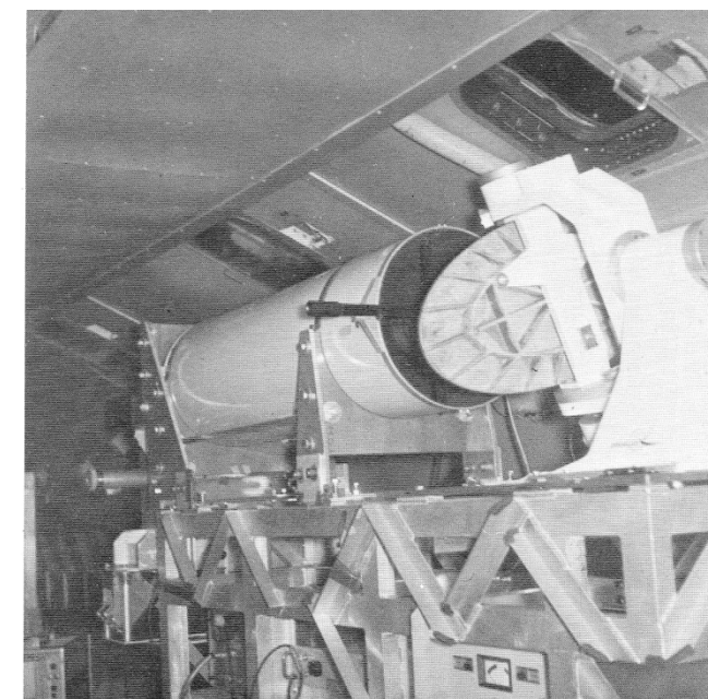
Kuiper and Forbes' Telescope and Spectrometer and NASA Heliostat Installed on the Convair 990
