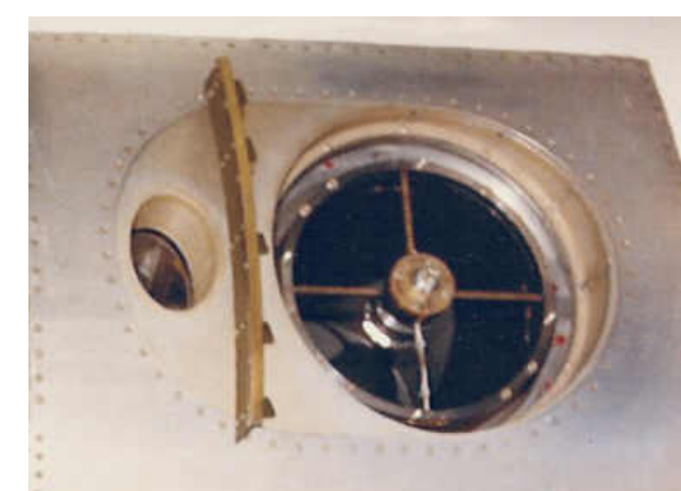
The gimbal-mounted telescope had a controlled-leak, a spherical air seal at the fuselage that permitted articulation.
