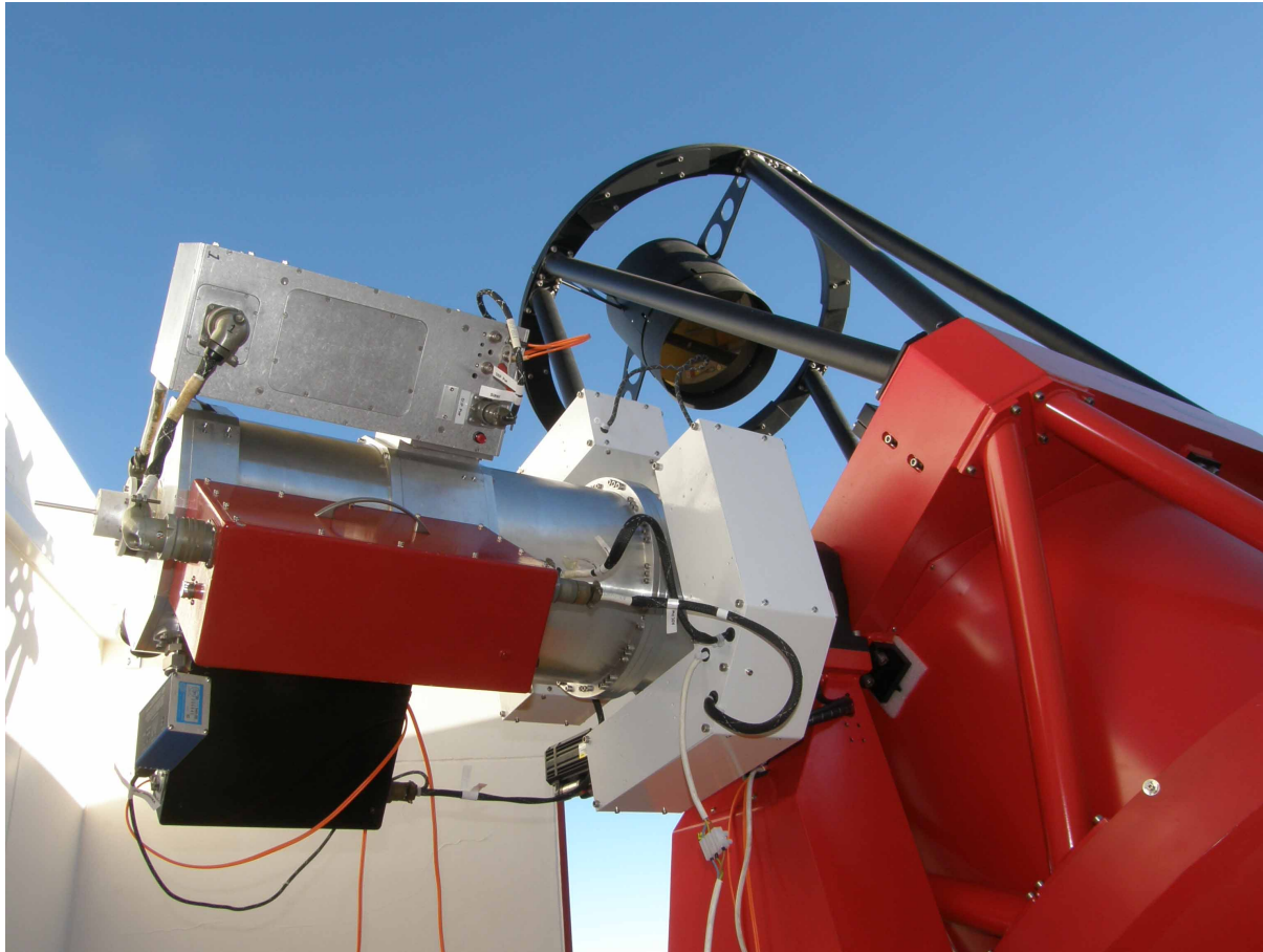
The IRIS telescope and IR camera in its enclosure at OCA IRIS is a collaborative project of AIRUB, IfA, and UCN 1K IR Camera on 0.8m telescope on Cerro Armazones, Chile
