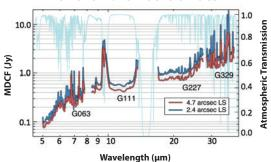
Grism continuum point source sensitivities for both wide and narrow long slits overlaid on an atmospheric transmission model (light blue). Values are for S/N = 4 in 900 s under nominal conditions.
