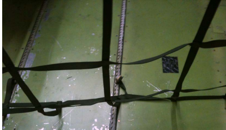
Figure 6.3-2: Telescope assembly barrier floor rail mounting points
