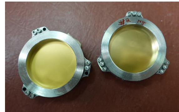
HIRMES fixed etalon imaging filters
