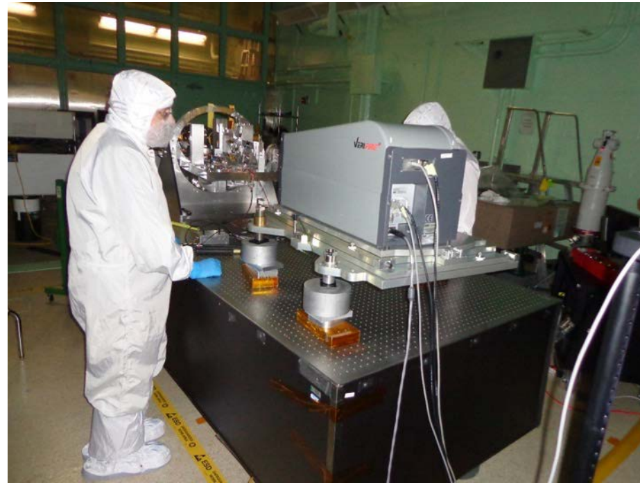
Aligning the Interferometer to HIRMES
