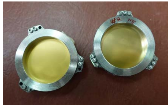
HIRMES fixed etalon imaging filters
