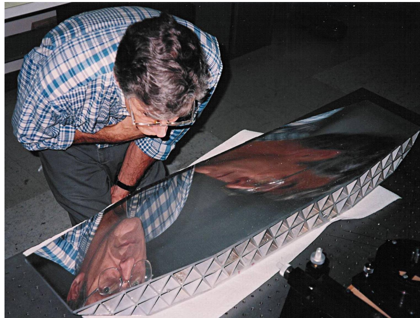
Figure 4. The AIRES echelle. Reflections are seen from both facets. From Erickson et al (2007)
