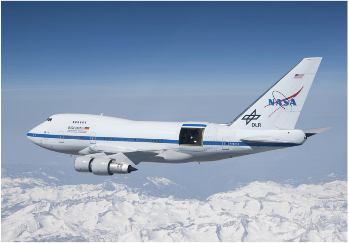
Figure 1. SOFIA flying over the Sierra Nevada mountains during an early test flight. The telescope door is open, though the mirror is under a protective cover. This image was taken by a NASA F-18 chase plane. In operations, SOFIA flies at night and provides otherwise unobtainable views of the universe at infrared wavelengths. (NASA/Jim Ross)
