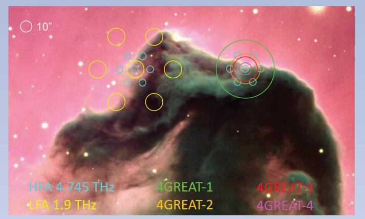
Transitioning from single pixels to pixel arrays and adding simultaneous multiple frequencies has transformed SOFIA/GREAT into an efficient mapping spectrometer. GREAT's beam-sizes (colors) and spatial configuration are superimposed on the Horsehead Nebula. For the 158 μm (1.9 THz) ionized carbon line, GREAT's mapping speed is ~50x faster than Herschel/HIFI to reach the same mapping sensitivity for an extended object (≥ few arcminutes).
