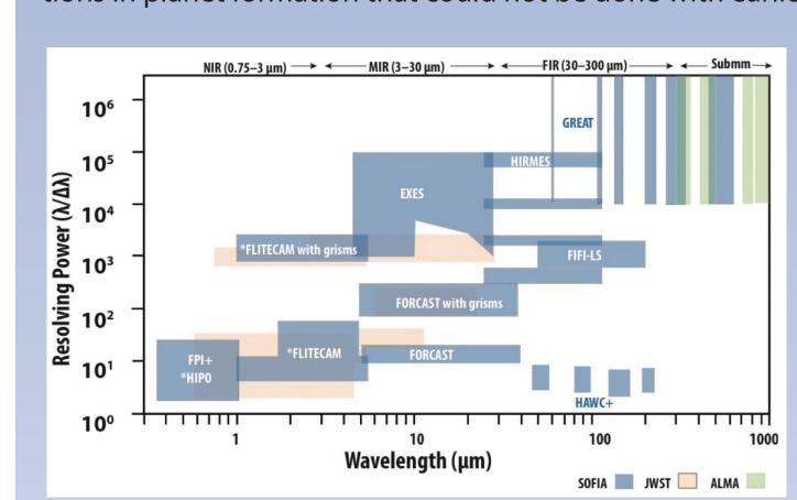
SOFIA instrumentation suite vs. resolution and wavelength coverage. SOFIA (blue boxes) complements ALMA and JWST. SOFIA's instruments fill the spectral gap between JWST's (orange) longest wavelength (28 μm) and ALMA's (green) shortest wavelength (320 µm). HIPO and FLITECAM were retired in Feb 2018. HIRMES becomes available in 2020.
