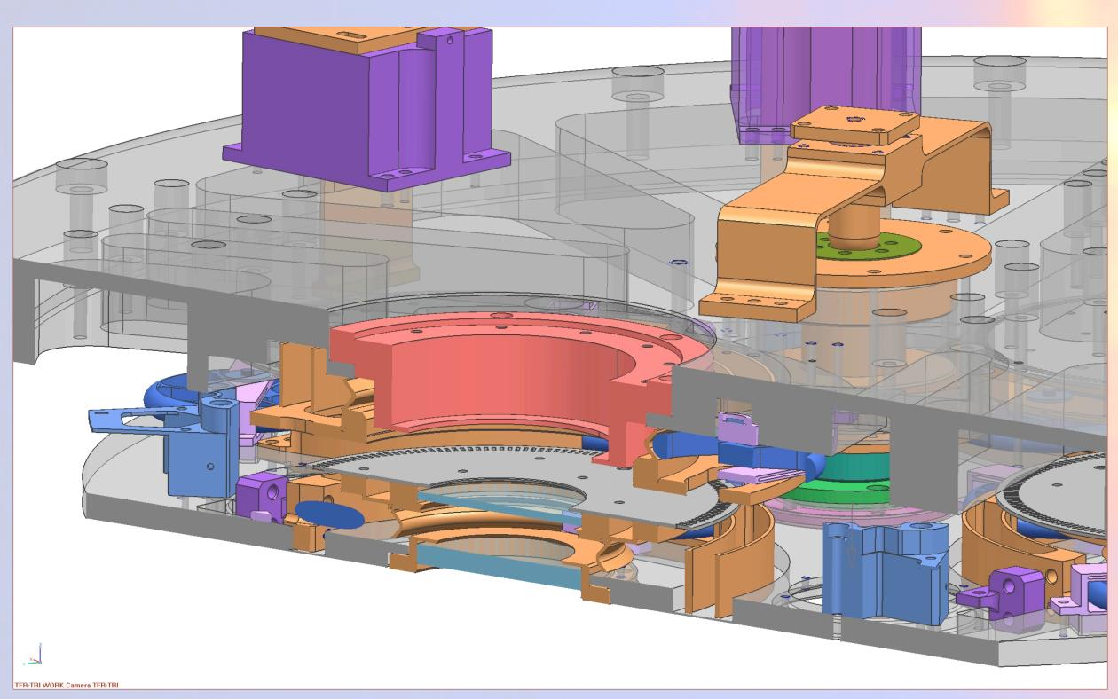
HAWCPol detects polarization with a slowly rotating quartz half-wave plate and fixed wire grid polarizer, both located in the pupil wheel. Components of HAWCPol have been demonstrated in the lab at cryogenic temperature, and we are currently assembling the full system over Summer 2010. The basic observing mode for HAWCPol is rapid (~10 Hz) chopping of the SOFIA secondary mirror, slow polarization modulation (~1 Hz), and occasional nodding of the telescope (~0.03 Hz).
