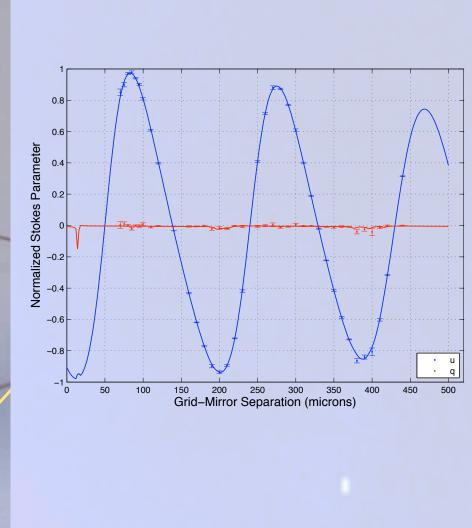
Left: The VPM consists of a polarizing grid in front of and parallel to a movable mirror. By varying the grid-mirror separation, the phase that is introduced between two orthogonal linear polarizations can be changed resulting in a modulation of the polarization state of the incoming radiation (Chuss et al. 2006). Right: Preliminary results are shown for a single VPM. The VPM modulates a single linear Stokes parameter as the grid-mirror separation is varied.
