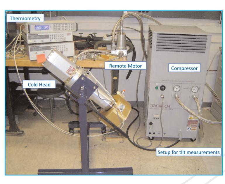
surface as a function of tilt angle have shown that a pule tube cooler can tilt up to  $\pm 30^{\circ}$  with very little degradation to its performance.
