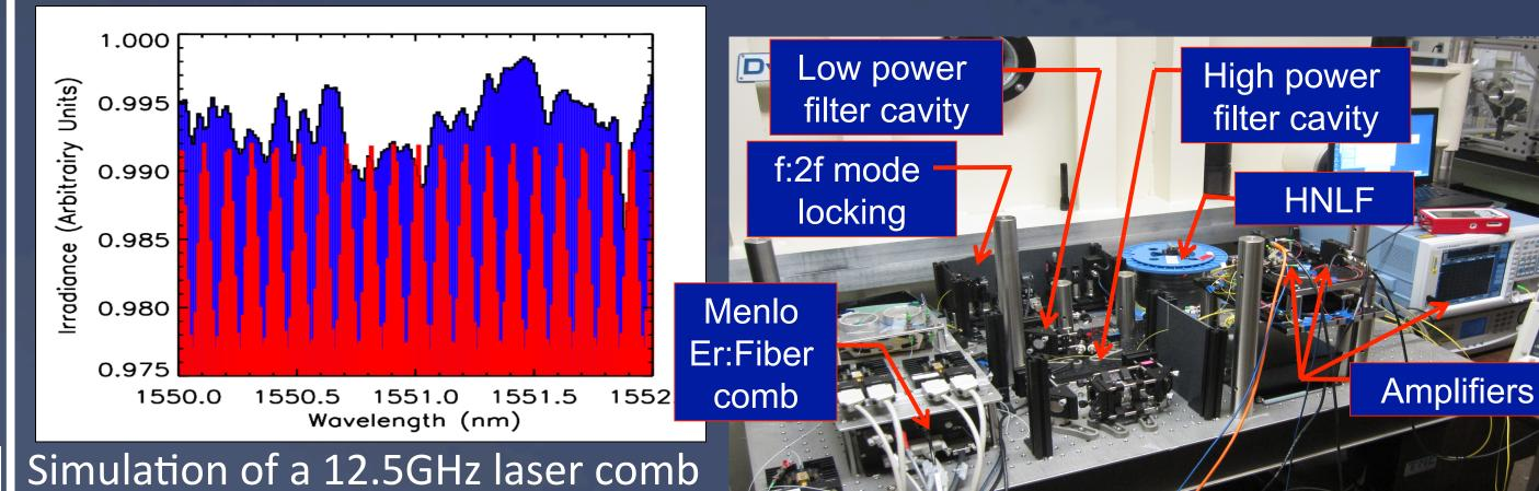
Simulation of a 12.5GHz laser combosine spectrum overlaid on an M6 spectrum at R=55,000. Comb + spectrograph  $\Rightarrow 5-7$ m/s precision. (M6 spectrum from Peng Jiang)
