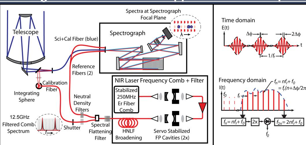
(right) Laser frequency comb functioning as both a simultaneous and overlaid wavelength reference. The laser comb is well suited for use with fiber fed systems. (left) The frequency comb spectrum is the Fourier transform of a pulse train with the group and phase velocities offset by  $\Delta \phi$ .  $f_0$  and  $f_r$  are RF and easily stabilized to high precision.
