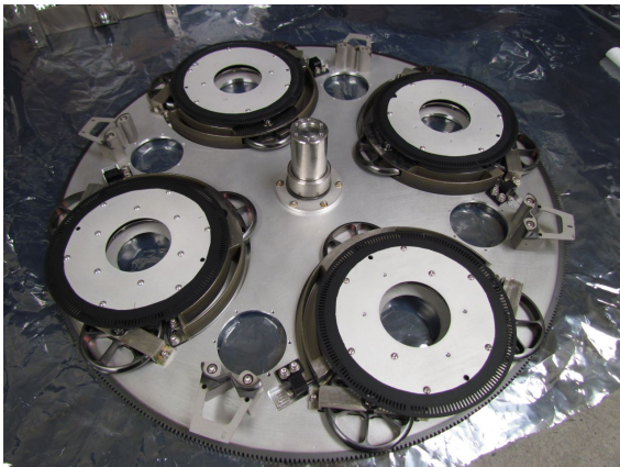
polarimeter (JPL, U. Illinois): in advanced state of development; continuous and stepped rotation of quartz half-wave plates
