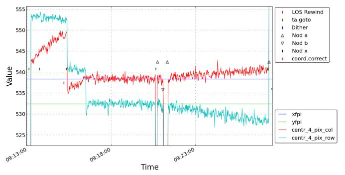
D. Hoffman - plot of Line Ops showing drift of asteroid Vesta from SIBS after pointing to a sidereal object during Line Ops
