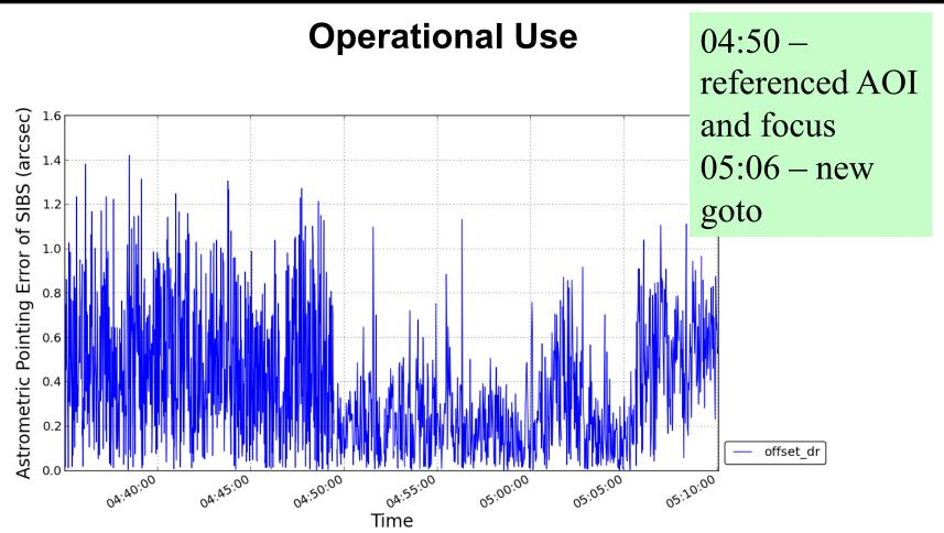
D. Hoffman - plot of astrometric pointing error while tracking on asteroid Pallas during flight 148.
