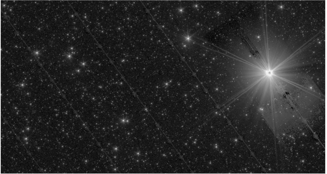
Figure 15: Example of latents (from the bright object on the right) in an IRAC [3.6] image (centered at l=165.2^\circ , b=-0.45^\circ ). There are also full array pull-ups near the bright source.
