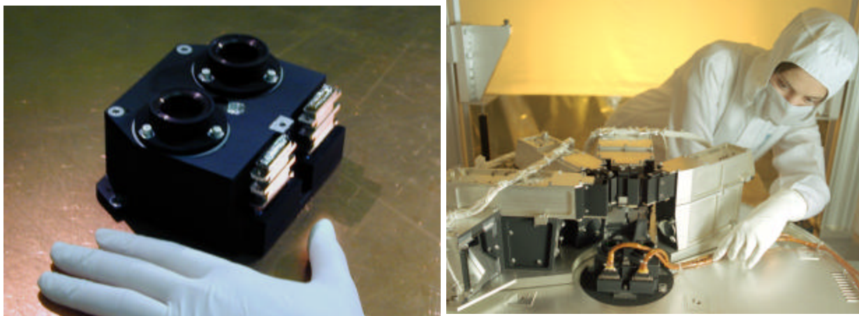
Figure 1a: The Flight Cold Assembly, on the bench and during its installation into the Multiple Instrument Chamber.
